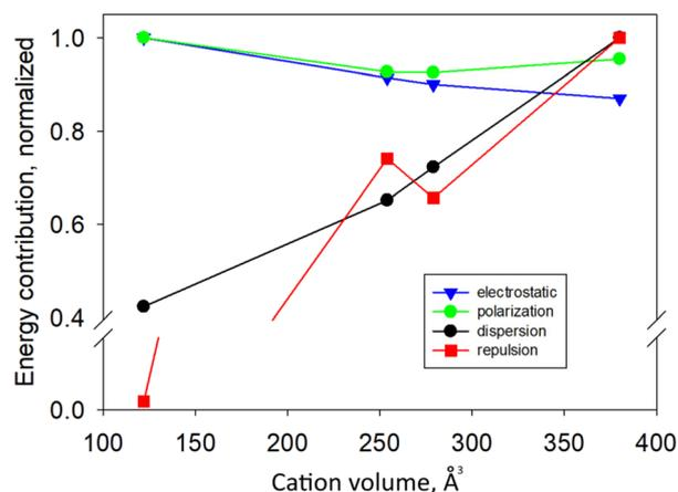
**Fig. 12** Plot of the energy contribution for each term (electrostatic, polarization, dispersion and repulsion) based on SDs for all complexes against the cation volume. Energies are normalized relative to those related to the largest cation (TBA) and averaged over the two highest SDs.
