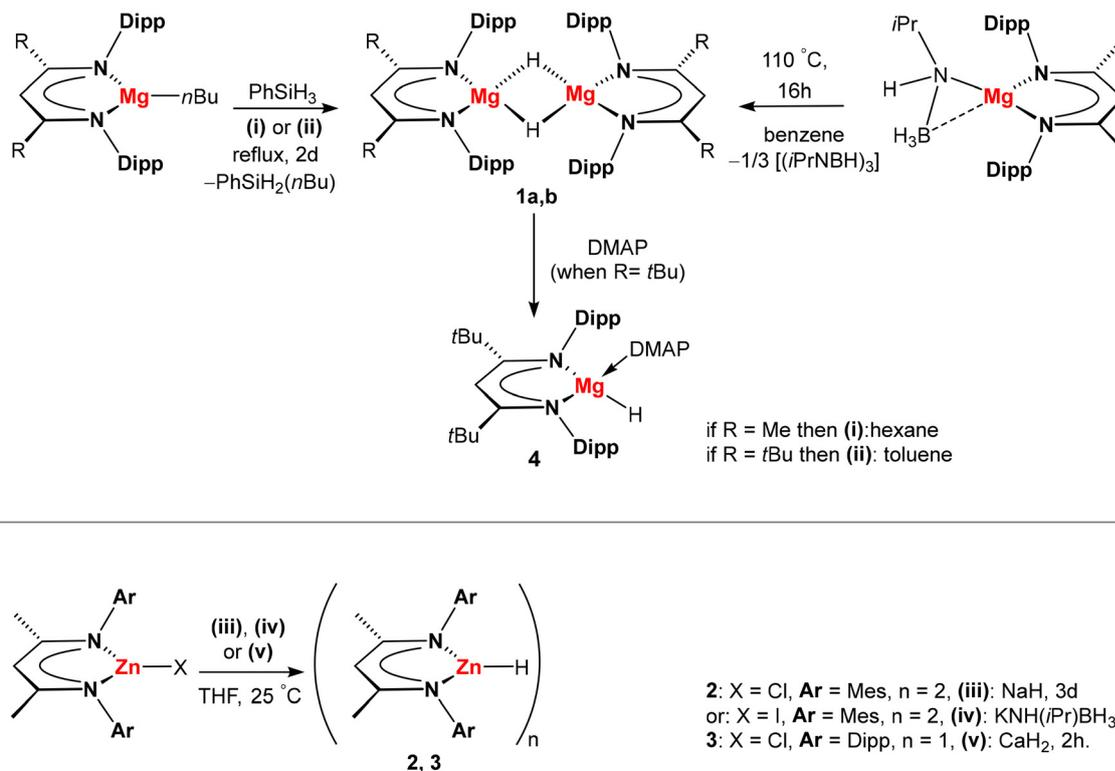
**Scheme 1** Synthesis of BDI-stabilised magnesium and zinc hydrides. Top: synthesis of dimeric magnesium hydrides **1a** (R = Me) by hydrosilane metathesis as well as  $\beta$ -hydride elimination routes, with **1b** (R = *t*Bu) and the monomeric magnesium hydride (**4**) as a DMAP adduct. Bottom: synthesis of dimeric and monomeric zinc hydrides **2** and **3**.
