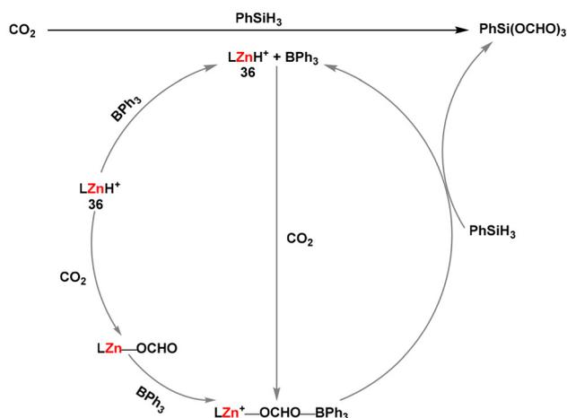
**Scheme 11** Proposed catalytic cycle for the selective hydrosilylation of CO<sub>2</sub> using PhSiH<sub>3</sub> in the presence of the hydrido zinc cation **36** and triphenylborane.
