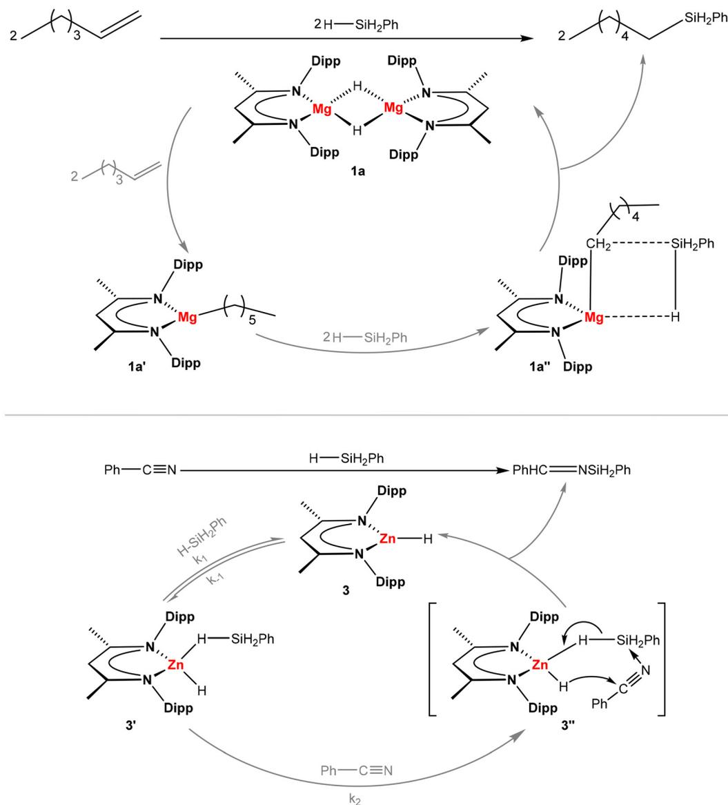
**Scheme 2** Proposed cyclic mechanisms for catalytic hydrosilylation (with PhSiH<sub>3</sub>) of (top) 1-hexene in the presence of **1a** and (bottom) benzonitrile in the presence of **3**.
