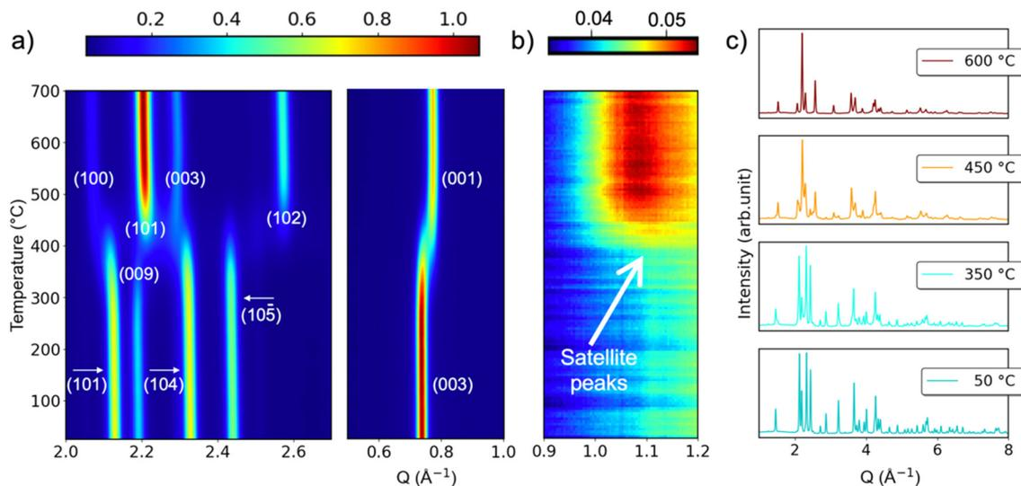
**Fig. 5** *In situ* SXPd of LuMnGaO<sub>4</sub> as it oxidizes. (a) Contour plots of *in situ* SXPd data for LuMnGaO<sub>4</sub> heated in air from 25 °C to 700 °C. (b) Enlarged view (magnified 20 $\times$ ) highlighting the appearance of satellite peaks. (c) Selected diffraction patterns at 50 °C, 350 °C, 450 °C, and 600 °C.
