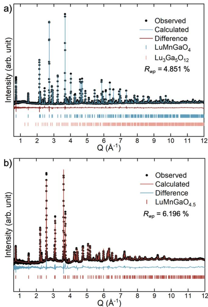
**Fig. 2** Neutron powder diffraction patterns with Rietveld fits for (a) the reduced phase,  $\text{LuMnGaO}_4$ , and (b) the oxidized phase,  $\text{LuMnGaO}_{4.5}$ . Data were collected using the POWGEN<sup>30</sup> instrument at the Spallation Neutron Source, Oak Ridge National Laboratory, with a center wavelength of 0.8 Å at 300 K.
