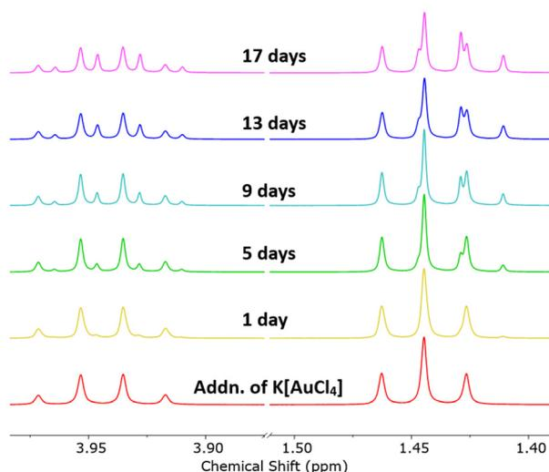
Fig. 9 Stacked plot of  $^1\text{H}$  NMR spectra in acetone- $\text{d}_6$  following the addition of  $\text{K}[\text{AuCl}_4]$  to  $[\text{Au}(\text{Et}_2\text{dtc})_2][\text{BF}_4]$  (red, bottom) at 4 day intervals.
