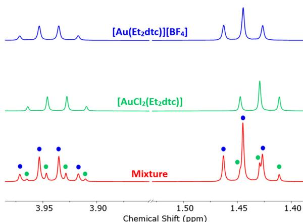
**Fig. 6** Portions of the  $^1\text{H}$  NMR spectra ( $\text{acetone-d}_6$ ) of  $[\text{Au}(\text{Et}_2\text{dtc})_2][\text{BF}_4]$  (blue, top);  $[\text{AuCl}_2(\text{Et}_2\text{dtc})]$  (green, middle) and the as-synthesized mixture which precipitated from water (red, bottom) with the coloured circles indicating which peaks correspond to which component of the mixture.
