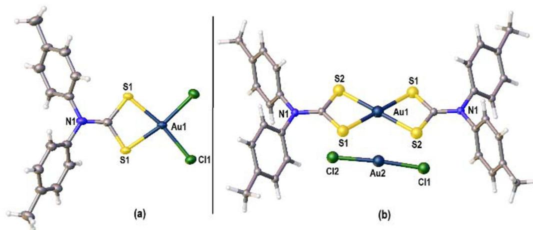
Fig. 5 Solid-state molecular structure of (a)  $[AuCl_2(p\text{-tolyl}_2dtc)]_2$ . Selected bond lengths: Au–Cl 2.3167(11), Au–S 2.2979(12) Å; (b)  $[Au(p\text{-tolyl}_2dtc)_2][AuCl_2]$ . Range of Au–S bond lengths (Å): 2.3326(6)–2.3399(6).
