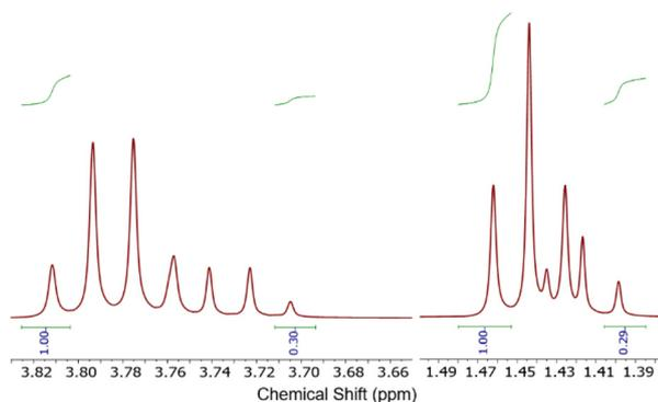
Fig. 3 The  $^1\text{H}$  NMR spectrum (in  $\text{CDCl}_3$ ) of the as-synthesized  $[\text{AuCl}_2(\text{Et}_2\text{dtc})]$  mixture focused on the  $\text{CH}_2$  and  $\text{CH}_3$  regions of the spectrum.
