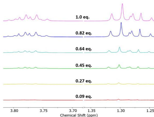
**Fig. 7** Stacked plot of  $^1\text{H}$  NMR spectra ( $\text{DMSO-d}_6$ ) following the portionwise addition of  $\text{Na}(\text{Et}_2\text{dtc})$  to  $\text{Na}[\text{AuCl}_4]$ . The majority product is  $[\text{Au}(\text{Et}_2\text{dtc})_2]^+$  and the minority product is  $[\text{AuCl}_2(\text{Et}_2\text{dtc})]$ .
