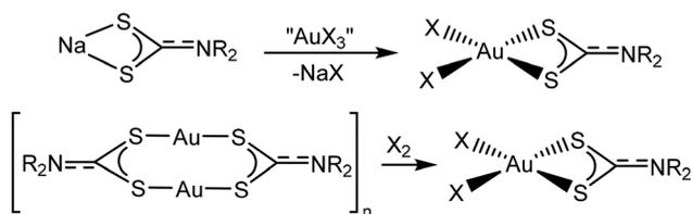
**Scheme 1** The two most common synthetic routes towards “[AuX<sub>2</sub>(dtc)]” by salt metathesis (top) and oxidative addition (bottom). X = Cl or Br; R<sub>2</sub> = dialkyl, cyclic alkyl, diaryl.
