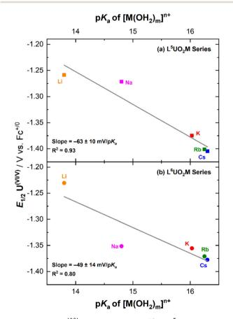
Fig. 7 Plot of  $E_{1/2}(U^{VI/V})$  vs.  $pK_a$  of  $[M(H_2O)_m]^{n+}$  for  $L^5UO_2M$  complexes (a, upper panel) and L<sup>6</sup>UO<sub>2</sub>M complexes (b, lower panel).
