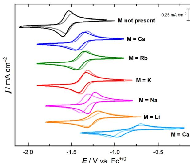
Fig. 6 *In situ* cyclic voltammetry experiments for uranium complexes used in this study.  $L^5UO_2$  and  $L^5UO_2M$  complexes are represented by solid colors;  $L^6UO_2$  and  $L^6UO_2M$  complexes are represented by faded colors. Electrolyte: 0.1 M TBAPF<sub>6</sub> in CH<sub>3</sub>CN, scan rate: 100 mV s<sup>-1</sup>, electrode: highly oriented pyrolytic graphite.
