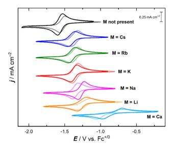
Fig. 6 In situ cyclic voltammetry experiments for uranium complexes used in this study. L<sup>5</sup>UO<sub>2</sub> and L<sup>5</sup>UO<sub>2</sub>M complexes are represented by solid colors; L<sup>6</sup>UO<sub>2</sub> and L<sup>6</sup>UO<sub>2</sub>M complexes are represented by faded colors. Electrolyte: 0.1 M TBAPF<sub>6</sub> in CH<sub>3</sub>CN, scan rate: 100 mV s<sup>-1</sup>, electrode: highly oriented pyrolytic graphite.
