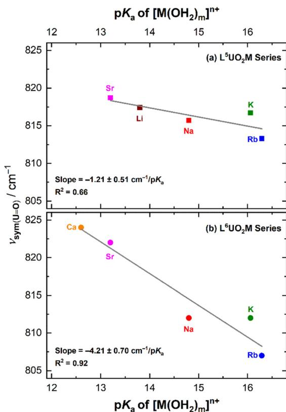
Fig. 8 Dependence of the U=O symmetric stretching frequency from Raman spectroscopy of the  $L^5UO_2M$  (a, upper panel) and  $L^6UO_2M$  (b, lower panel) complexes on the Lewis acidity ( $pK_a$ ) of the corresponding metal cation aqua complexes.
