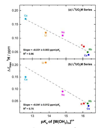
Fig. 10 Plots of  $\Delta \delta_{\max}^{1} H$  vs.  $pK_a$  of  $[M(H_2O)_m]^{n+}$  for  $L^5UO_2M$  complexes (a, upper panel) and L<sup>6</sup>UO<sub>2</sub>M complexes (b, lower panel).
