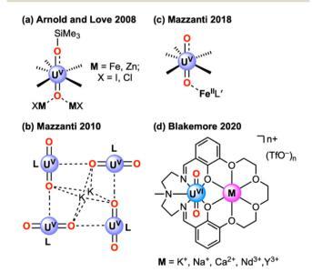
Fig. 1 Structures of complexes in which secondary cations influence the measured or apparent redox properties of the uranyl motif. From ref. 17a. 18 and 10.
