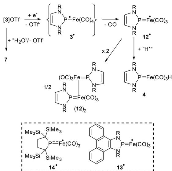
**Scheme 4** Proposed pathway for the formation of the products of the reactions of [3]OTf with LDA and reductants (Li, Cp<sub>2</sub>Co) and molecular structures of previously reported radicals 13<sup>•</sup> (ref. 19) and 14<sup>•</sup> (ref. 20) with similar molecular structure as 12<sup>•</sup>. Note that 7 can also arise from the hydrolysis of any of the products shown (R = Dipp).
