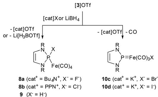
**Scheme 3** Reactions of [3]OTf with halide salts and LiBH<sub>4</sub> to furnish either diazaphospholene complexes (**8a,b, 9**) or NHP iron halides (**10c,d**) (R = Dipp, PPN = bis(triphenylphosphine)iminium).
