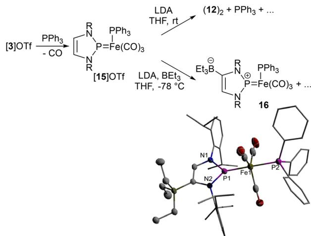
**Scheme 5** Synthesis of [15]OTf, its reaction with LDA under different conditions, and representation of the molecular structure of **16** in the crystal. For clarity, hydrogen atoms were omitted and the atoms in peripheral substituents drawn using a wire model. Thermal ellipsoids are drawn at the 50% probability level ( $R = \text{Dipp}$ ).
