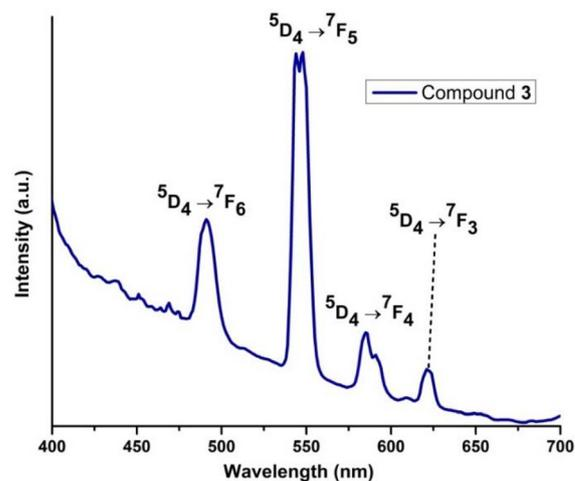
Fig. 8 Room-temperature solid-state emission spectrum for complex 3 excited at 360 nm.
