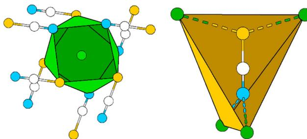
**Fig. 6** Excerpt of the crystal structure of  $\text{Pb}[\text{SCN}]_2$ . Left: distorted tetragonal antiprism around Pb (green). Right: distorted heterodisphenoid around  $[\text{SCN}]^-$  (yellow). Green: Pb, white: C, blue: N, yellow: S.
