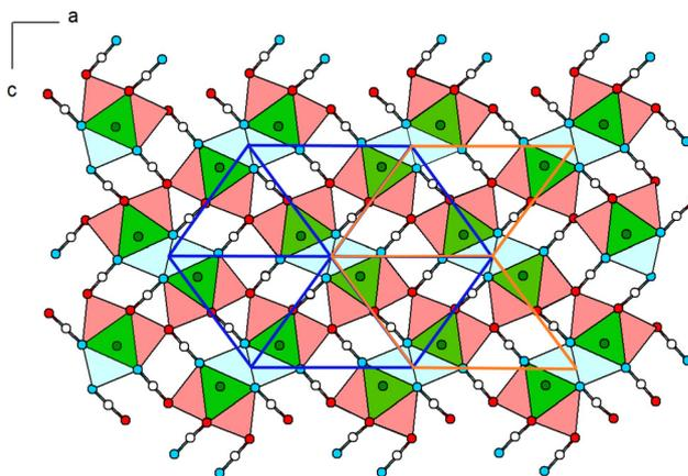
Fig. 3 Extended crystal structure of Pb[OCN]<sub>2</sub> viewed along [010]: coordination polyhedra around Pb (green, capped by O in red and N in blue) are connected *via* common [OCN]<sup>−</sup> anions and O atoms. The polyhedra form a monoclinic packing (outlined in orange), which can be interpreted as a distorted hexagonal rod packing (blue). Green: Pb, white: C, blue: N, red: O.
