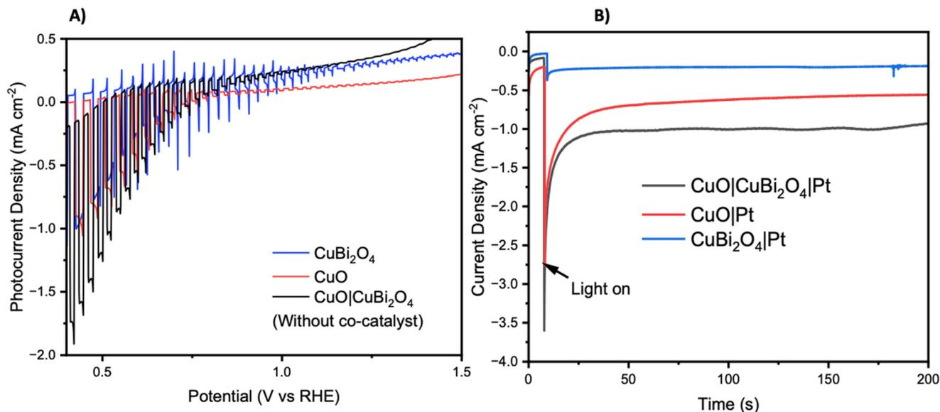
**Fig. 3** Photoelectrochemistry of unprotected photocathodes. (A) Chopped light linear sweep voltammetry of CuO, CuBi<sub>2</sub>O<sub>4</sub>, CuO|CuBi<sub>2</sub>O<sub>4</sub> at 10 mV s<sup>-1</sup> scanning from positive to negative. (B) Chronoamperometry under constant illumination at 0.4 V vs. RHE. Photo experiments were carried out using a Xe arc lamp calibrated to 1 sun (AM1.5G, 100 mW cm<sup>-2</sup>).
