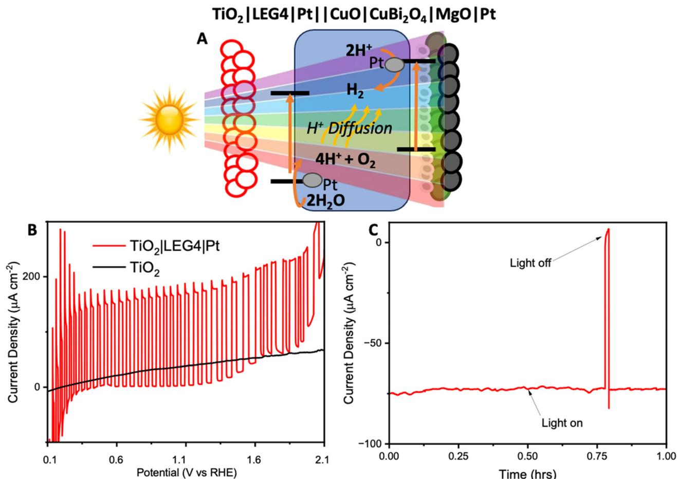
Fig. 5 Photoelectrochemistry of the bias-free tandem. (A) An illustration of the mechanism within the tandem upon illumination. (B) Chopped light linear sweep voltammetry of  $\text{TiO}_2$  (black) and  $\text{TiO}_2$  sensitized with LEG4 and Pt (red). (C) Chronoamperometry under no bias and constant illumination with 1 sun (Xe lamp, AM1.5G,  $100 \text{ mW cm}^{-2}$ ) for 1 hour.
