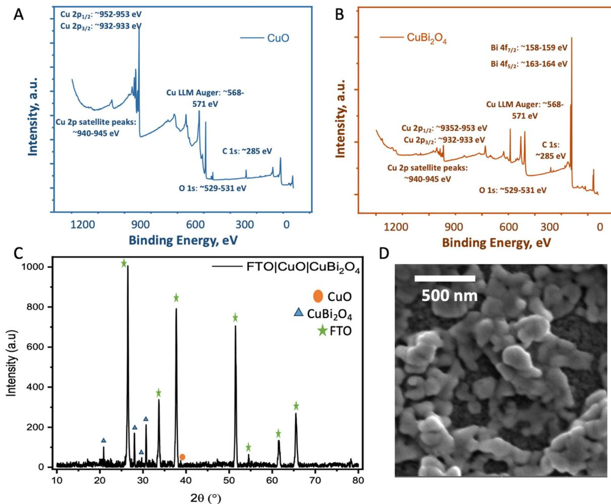
**Fig. 2** Physicochemical characterization. (A and B) XPS survey scans of CuO showing Cu 2p, O 1s and CuBi<sub>2</sub>O<sub>4</sub> (top) showing the Cu 2p, O 1s and Bi 4f peaks. (C) XRD of FTO|CuO|CuBi<sub>2</sub>O<sub>4</sub>. (D) SEM image of the CuO|CuBi<sub>2</sub>O<sub>4</sub> electrodes. The parameters of the SEM images are given in Fig. S5.†
