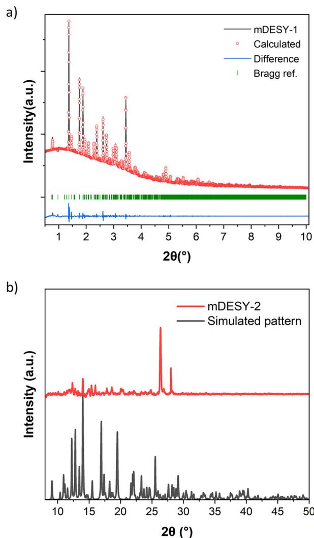
**Fig. 4** (a) PXRD of mDESYS-1 and Le Bail fit of the structure model from single crystal data on PXRD data collected at P02.1, PETRA III ( $\lambda = 0.20734$  Å), and (b) PXRD of mDESYS-2 collected in Bruker D8 Discover ( $\lambda = 1.5406$  Å) alongside its corresponding simulated pattern generated by the software Mercury.
