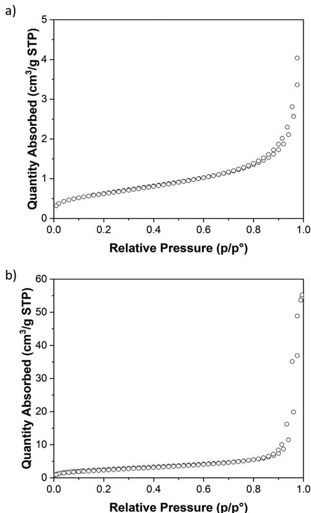
Fig. 6 N<sub>2</sub> adsorption measurements at 77 K of (a) mDESYS-1 and (b) mDESYS-2.
