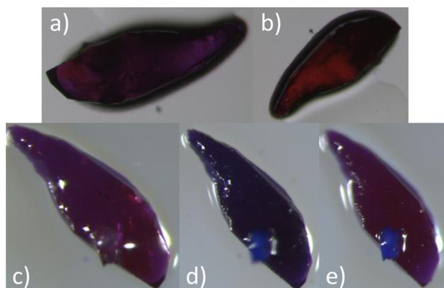
**Fig. 9** (a) and (b) Optical images of Azo@mDESYS-1 at room temperature at two different orientations in transmission mode. Optical images at different temperatures in reflectance mode: (c) room temperature, (d) 130 °C and (e) 2 h room temperature after heating at 130 °C.
