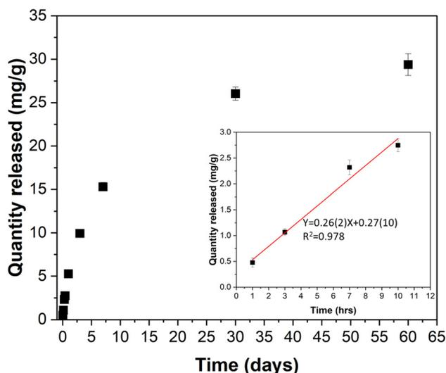
**Fig. 10** Release of azobenzene from mDESYS-1 in ethanol. Inset: Release of azobenzene during the first 10 h and its linear fitting.
