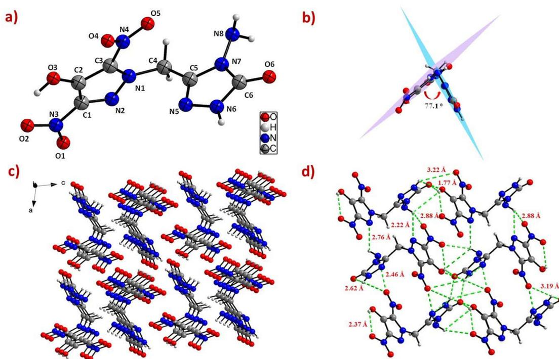
**Fig. 4** (a) Thermal ellipsoid plot (50%) and labelling scheme for **8**. (b) Dihedral angle between the pyrazole and triazolone ring. (c) Ball and stick packing diagram showing planar stacking in the crystal of **8** viewed along *b* axis. (d) Amplification of hydrogen bonding distribution in **8**.
