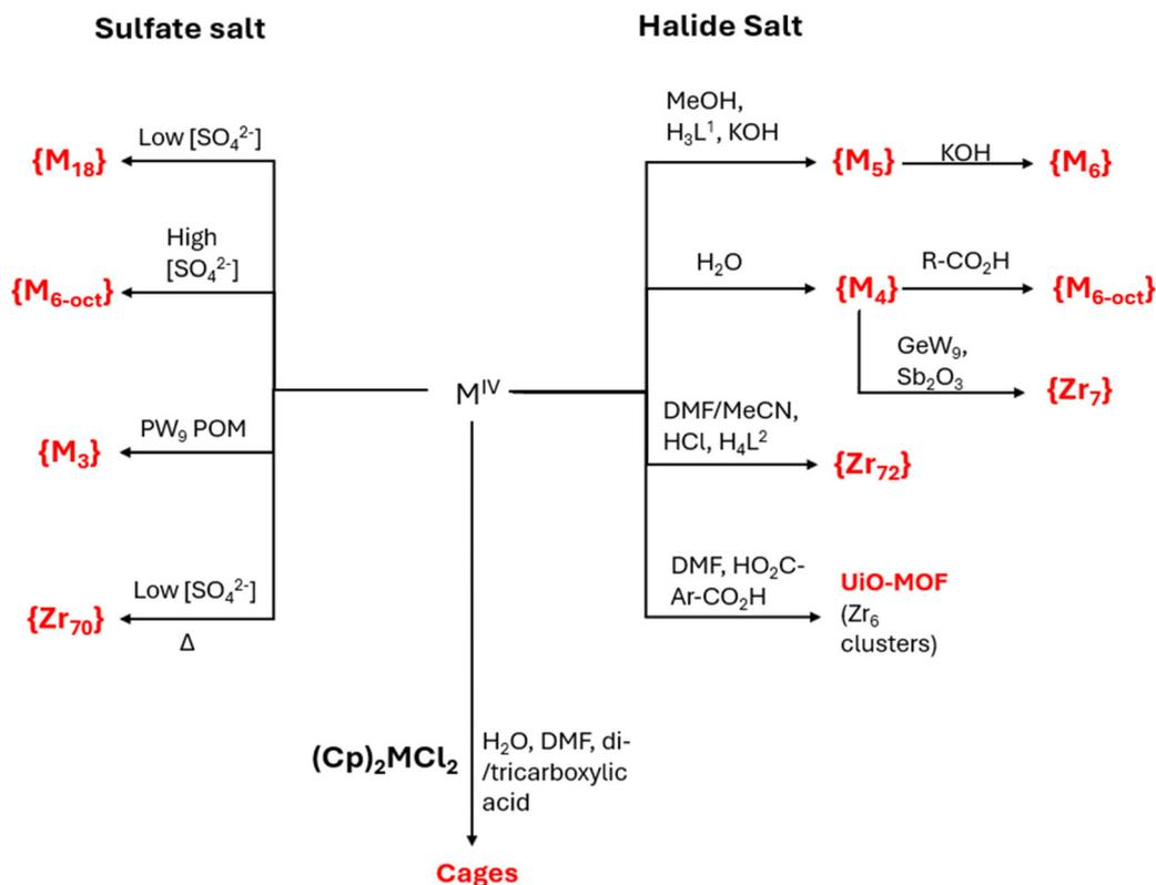
**Fig. 19** Schematic diagram of the reaction path towards Zr/Hf clusters discussed in this article. The reaction path is applicable to both Zr(IV) and Hf(IV), (M = Zr, Hf), unless otherwise stated. L<sup>1</sup> can be either H<sub>3</sub>dihydro or H<sub>3</sub>pidiox, L<sup>2</sup> is 3,3',3'',3'''-(anthracene-9,10-diylidenebis(methane-1,1-diyl-1-ylidene))tetrabenzoic acid.
