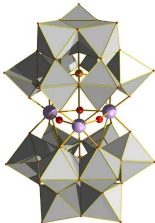
**Fig. 25** Polyhedral representation of  $[M_3(OH)_3]^{9+}$  cluster sandwiched between two tri-lacunary Keggin POMs.  $M = \text{Zr, Hf}$ . Keggin =  $[A-\alpha\text{-PW}_9\text{O}_{34}]^{9-}$ . Colour code: W, grey; P, orange; Zr, light purple; O, red. The Hf congener is isostructural.
