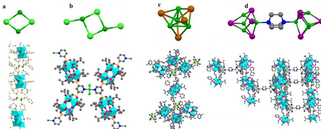
**Fig. 9** (a)  $\{Cu_2Cl_2\}$  doped 1D Ti–O material, (b)  $\{Cu_4Cl_4\}$  doped 2D material, (c)  $\{Cu_4Br_4\}$  doped 3D material, (d)  $\{Cu_4I_4\text{-DABCO-Cu}_4I_4\}$  doped 3D material. Hydrogens are omitted for clarity. Colour code: Ti, cyan; Cu, green; Cl, light green; Br, brown; I, purple; P, pink; S, yellow; C, grey; O, red; N, blue. This figure has been adapted/reproduced from ref. 66 with permission from American Chemical Society, copyright 2017.
