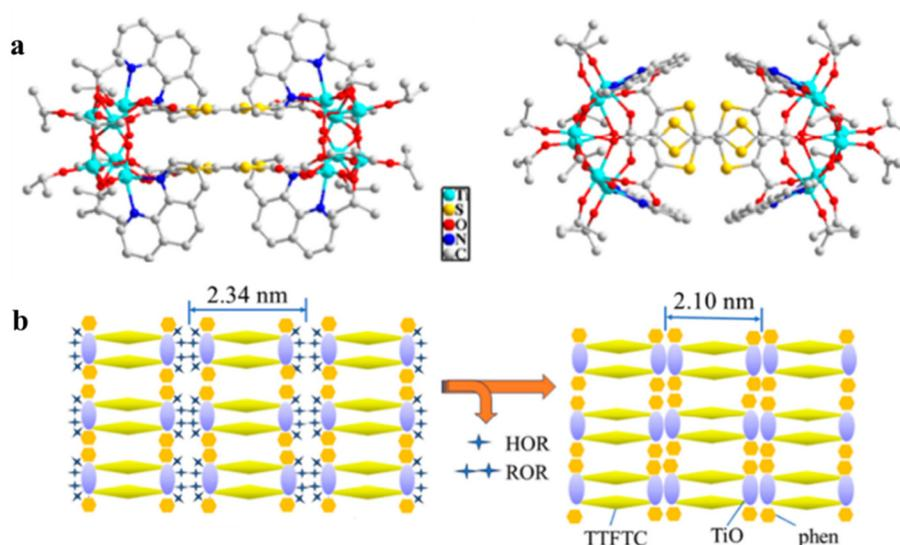
**Fig. 16** (a) The structure of  $[\text{Ti}_6\text{O}_6(\text{O}^i\text{Pr})_8(\text{TTFTC})(\text{phen})_2]_2$ . (b) TOC-MOF formed by condensation of isopropanol groups. Hydrogen atoms are omitted for clarity. This figure has been adapted/reproduced from ref. 89 with permission from American Chemical Society, copyright 2024.
