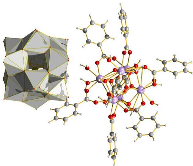
**Fig. 26** The co-crystallisation of a  $\text{Zr}_6$  benzoate with a silicotungstate Keggin POM showed synergistic enhancements in photochemical properties. The crystallisation resulted in ionic channels in the bulk structure, which the authors note as being a key aspect of its properties in photocatalysis.
