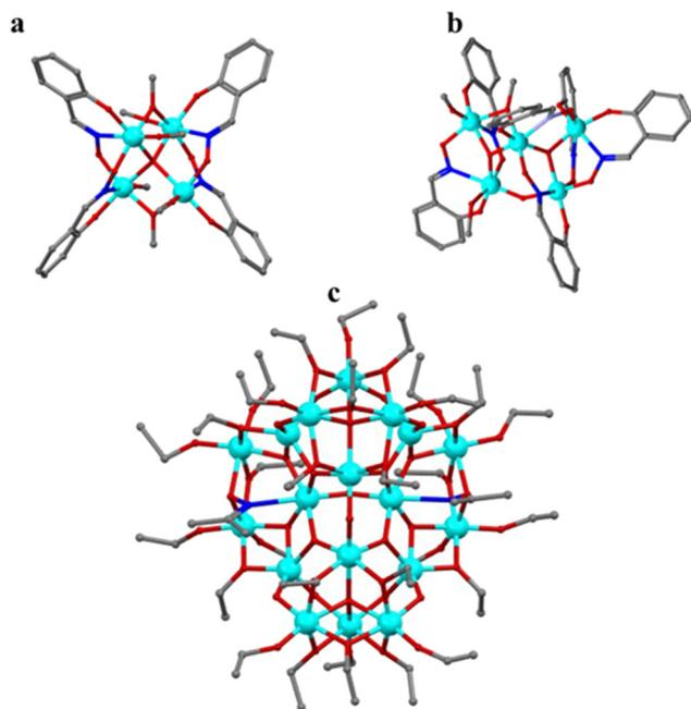
Fig. 5 Oxime-substituted titanium-oxo clusters: (a)  $Ti_4$ , (b)  $Ti_5$ , (c)  $Ti_{18}$ . Hydrogen atoms are omitted for clarity. Colour code: Ti, cyan; O, red; N, blue; C, grey.
