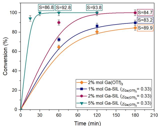
**Fig. 11** Performance of various amounts of Ga-SIL ( $\chi_{\text{Ga}(\text{OTf})_3} = 0.33$ ) in the [3 + 3] cycloaddition of 2,4-dimethylphenol to isoprene, relative to metal triflate. Reaction conditions: 2,4-dimethylphenol (8 mmol), isoprene (4 mmol), 1000 rpm,  $T = 35^\circ\text{C}$ ,  $S$  – selectivity to the main product.
