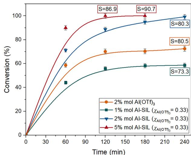
**Fig. 10** Performance of various amounts of Al-SIL ( $\chi_{\text{Al}(\text{OTf})_3} = 0.33$ ) in the [3 + 3] cycloaddition of 2,4-dimethylphenol to isoprene, relative to metal triflate. Reaction conditions: 2,4-dimethylphenol (8 mmol), isoprene (4 mmol), 1000 rpm,  $T = 35^\circ\text{C}$ ,  $S$  – selectivity to the main product.
