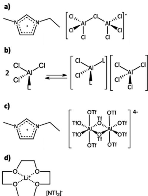
**Fig. 1** Examples of the structures of metal-containing ionic liquids: (a) chlorometallate ionic liquid, (b) liquid coordination complex (LCC),<sup>3</sup> (c) trifluoroaluminate ionic liquid,<sup>8</sup> and (d) solvate ionic liquid.<sup>14</sup>
