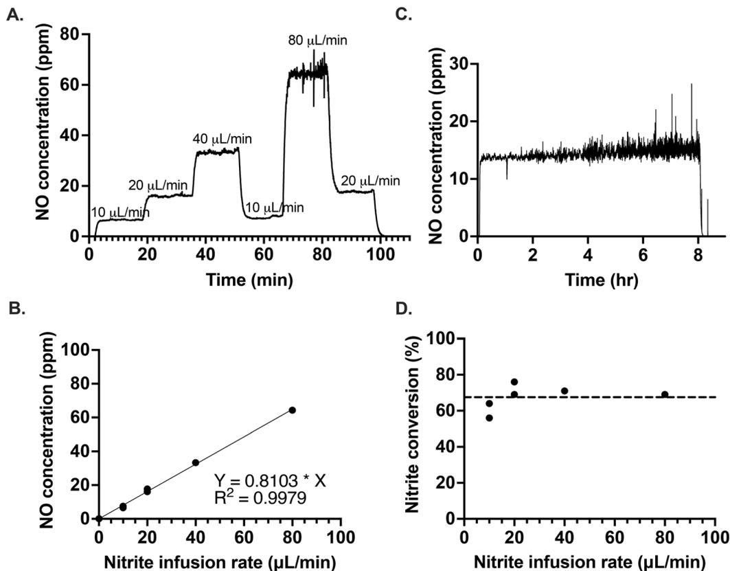
**Fig. 3** Control of NO generation by the variation of nitrite infusion rate into a solution of  $[\text{Cu}(\text{I})\text{L}]\text{SO}_4$  (7 mM) and calcium ascorbate (140 mM); (A) 10–80  $\mu\text{L min}^{-1}$   $\text{NaNO}_2$ , (B) correlation between the nitrite infusion rate and the concentration of NO generated, (C) 7.2 mL of 10 mM  $\text{NaNO}_2$  at 15  $\mu\text{L min}^{-1}$ , (D) average (dashed line) conversion as a function of nitrite infusion rate.
