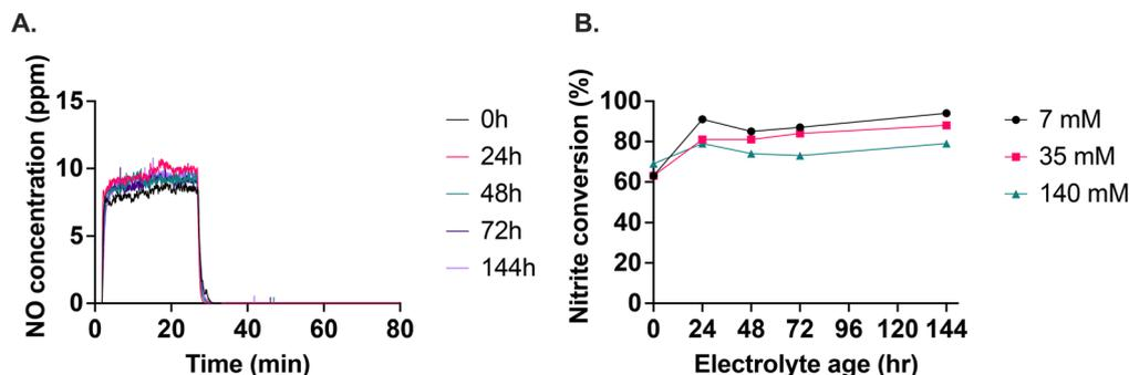
**Fig. 4** Effect of storage on the optimized electrolyte (A). A total of 250  $\mu\text{L}$  of 10 mM  $\text{NaNO}_2$  was infused at 10  $\mu\text{L min}^{-1}$  into electrolyte stored over time. (B) Nitrite conversion to NO as a function of calcium ascorbate concentration over six days.
