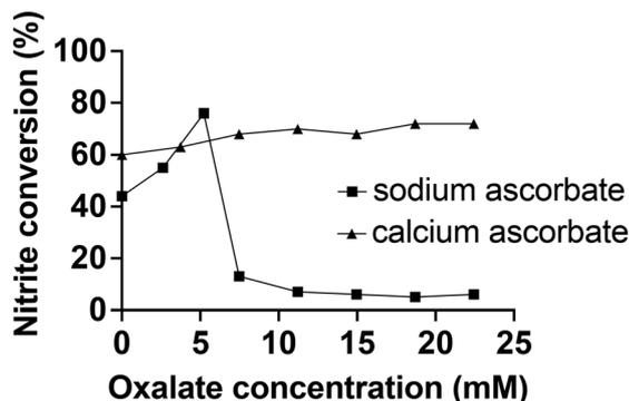
Fig. 5 The effect of oxalate concentration on nitrite conversion to NO.  $15 \mu\text{L min}^{-1}$  of nitrite was infused to 5 mL of electrolyte containing either 280 mM sodium ascorbate or 140 mM calcium ascorbate. The titration was performed by bolus injections of 100  $\mu\text{L}$  of 187 mM sodium oxalate in MES pH 5.8 into the electrolyte.
