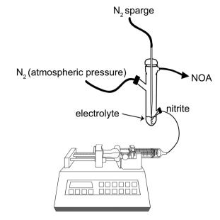
Fig. 2 Schematic of the experimental setup for NO generation through nitrite infusion into electrolyte.
