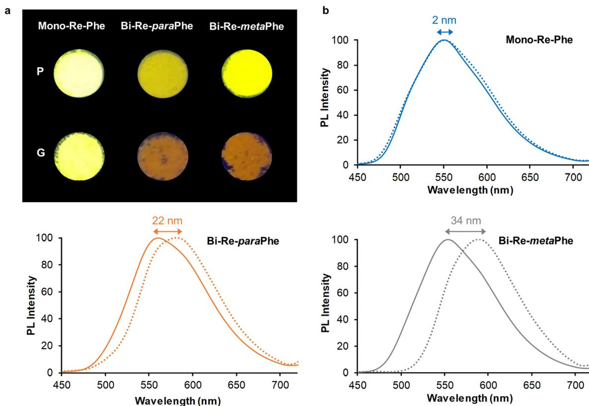
**Fig. 8** (a) Image of the pristine and ground powders of the three complexes illuminated by UV light at 365 nm. (b) Normalized photoluminescence spectra of **Mono-Re-Phe** (blue lines), **Bi-Re-paraPhe** (orange lines), and **Bi-Re-metaPhe** (grey lines), as microcrystalline pristine powders (solid lines) and ground powders (dotted lines). The wavelength shift between maxima is indicated. Excitation at 380 nm.
