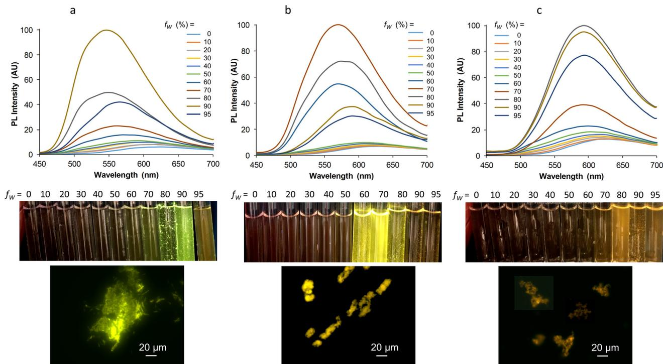
**Fig. 9** From top to bottom: emission spectra of **Mono-Re-Phe** (a), **Bi-Re-paraPhe** (b), and **Bi-Re-metaPhe** (c) at  $\sim 1.5 \times 10^{-5}$  M in acetonitrile solutions containing from 0 to 95% water,  $\lambda_{\text{ex}} = 364$  nm; corresponding samples illuminated at 365 nm; fluorescence microscopy images of the suspensions at  $f_w = 80\%$  or  $90\%$ . All samples were observed 3 h after preparation.
