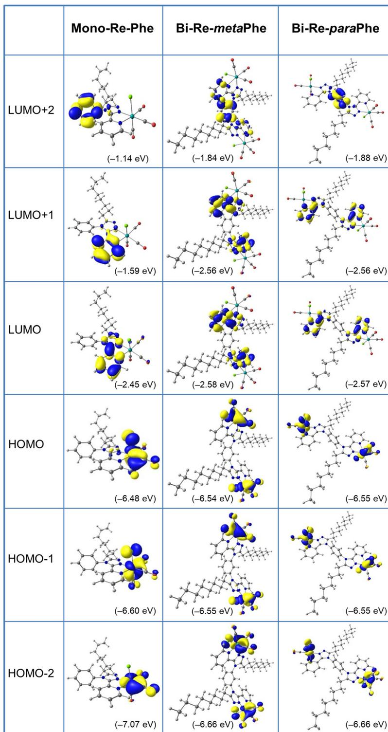
Fig. 5 Isodensity plots (isovalue = 0.03 e bohr<sup>-3</sup>) and energy levels of the first frontier molecular orbitals, for complexes **Mono-Re-Phe**, **Bi-Re-*para*Phe**, and **Bi-Re-*meta*Phe** in dichloromethane, according to DFT calculations at the PBE1PBE/LANL2DZ level of theory.
