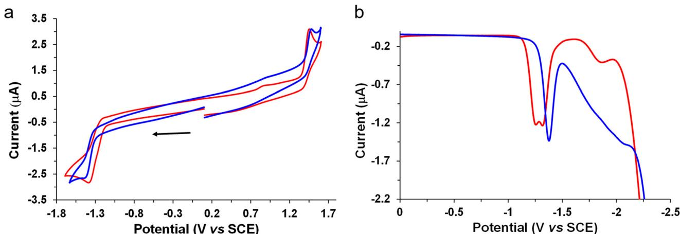
**Fig. 6** (a) Cyclic voltammograms of the first oxidation and reduction processes of complexes **Mono-Re-Phe** ( $2 \times 10^{-3}$  M, blue line) and **Bi-Re-*para*Phe** ( $1 \times 10^{-3}$  M, orange line) at  $0.2 \text{ V s}^{-1}$  (left); (b) their OSWVs cathodic scans (right) on a Pt working electrode in  $\text{CH}_2\text{Cl}_2 + 0.1$  M  $n[\text{Bu}_4\text{N}][\text{BF}_4]$  at room temperature.
