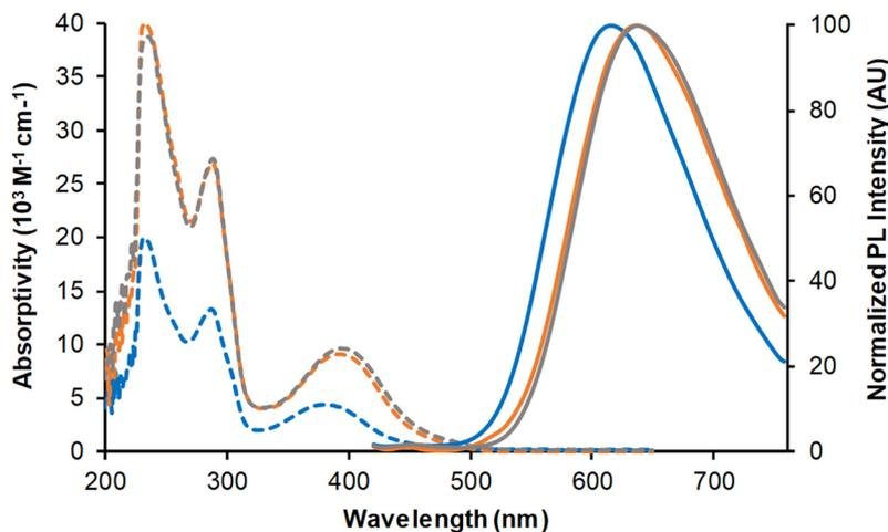
**Fig. 7** UV-vis absorption spectra (dotted lines) and normalized emission spectra (solid lines) of complexes **Mono-Re-Phe** (blue lines), **Bi-Re-paraPhe** (orange lines), and **Bi-Re-metaPhe** (grey lines) in aerated dichloromethane. Concentrations:  $\sim 5 \times 10^{-5}$  M (monomer) and  $2.5 \times 10^{-5}$  M (dimers) for absorption,  $\sim 1.1 \times 10^{-5}$  M (monomer) and  $5.1 \times 10^{-6}$  M (dimers) for emission. Excitation in the low-energy absorption band.
