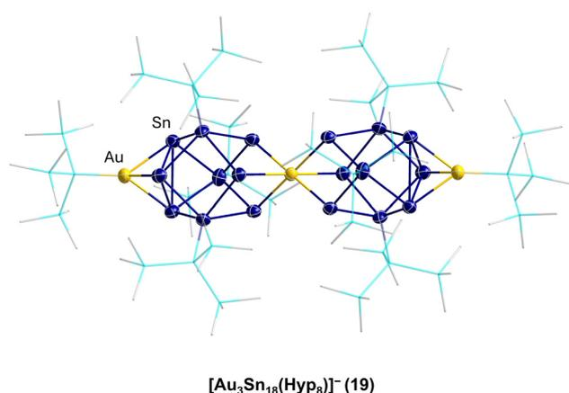
**Fig. 4** First use of the [Sn<sub>9</sub>Hyp<sub>3</sub>]<sup>-</sup> cage as a ligand in coordination chemistry to form **19**. Ligands are simplified by wires and sticks, and hydrogen atoms are omitted for clarity (light blue = silicon, light grey = carbon, yellow = gold, and dark blue = tin).
