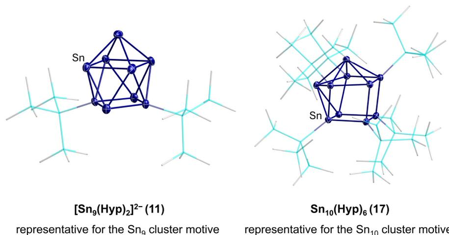
**Fig. 3** Examples for metalloids clusters synthesized *via* the disproportionation reaction. Ligands are simplified by wires and sticks, hydrogen atoms are omitted for clarity (light blue = silicon, light grey = carbon, and dark blue = tin).
