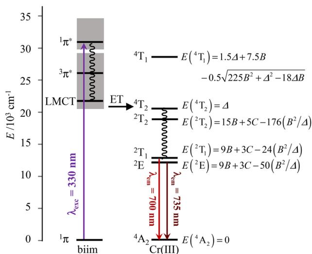
**Fig. 5** Jablonski diagram of homoleptic  $[\text{Cr}(\text{H}_2\text{biim})_3]^{3+}$  or  $[\text{Cr}(\text{Me}_2\text{biim})_3]^{3+}$  complexes showing the antenna effect upon UV excitation at 330 nm. The modeling of the energies of the Cr levels is taken from ref. 64.
