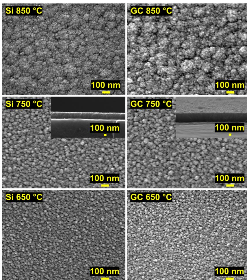
**Fig. 7** Top view SEM images of ZrN on Si (left) and GC (right) deposited at 850 °C (top), 750 °C (middle) and 650 °C (bottom). Cross section images of the film deposited at 750 °C are shown in the inset.
