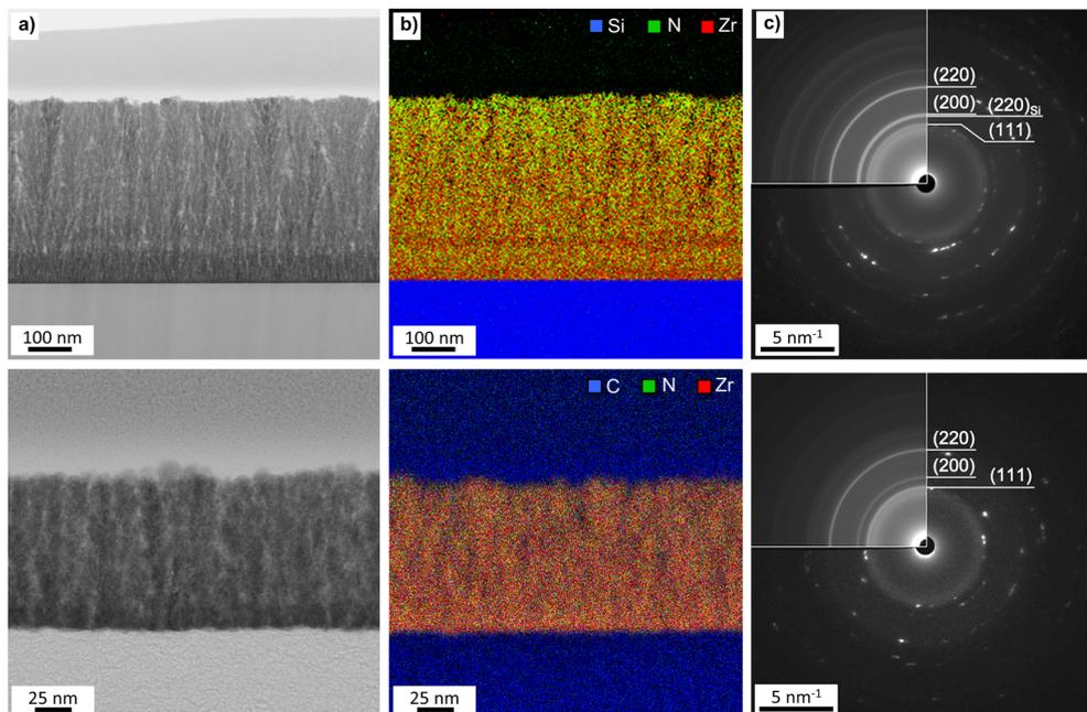
**Fig. 8** (a) BF-TEM, (b) STEM-EDS and (c) SAED of ZrN deposited at 750 °C on Si (top) and GC (bottom). Rotational averaging (inserts) is used in the identification of both diffracted planes. The patterns are indexed as ZrN using inorganic crystal structures data from ICSD-131632 (ICSD release 2021 02 01).<sup>38,39</sup>
