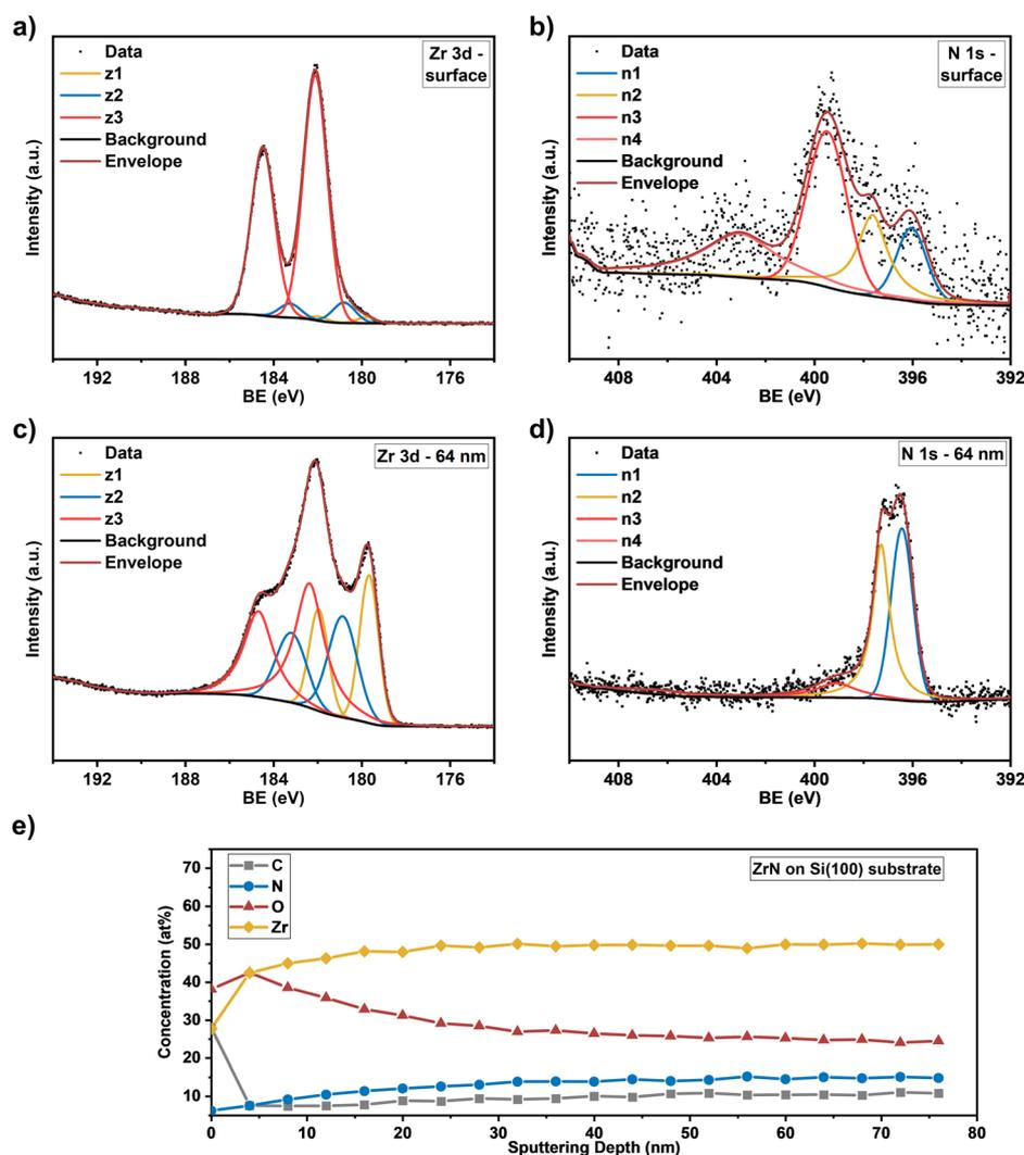
Fig. 5 High resolution core level spectra of (a) Zr 3d at the surface and (c) at a sputtering depth of 64 nm and (b) N1s at the surface and (d) at a sputtering depth of 64 nm for the ZrN film. (e) Concentration profile of the elements (Zr, N, O, C) as a function of sputtering depth on the Si(100) substrate.
