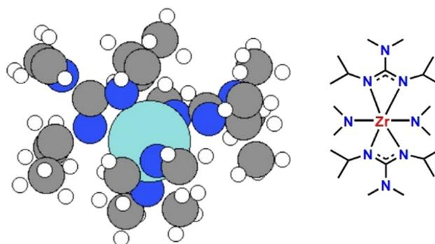
**Fig. 1** The configuration of SSP [Zr(guan)<sub>2</sub>(NMe<sub>2</sub>)<sub>2</sub>] (1) (right) used to deposit ZrN. The left image shows a 3D structure of the precursor in which Zr is the large cyan sphere, nitrogen the blue spheres, carbon grey spheres and hydrogen white spheres.
