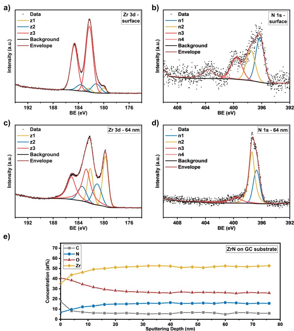
Fig. 4 High resolution core level spectra of (a) Zr 3d at the surface and (c) at a sputtering depth of 64 nm and (b) N 1s at the surface and (d) at a sputtering depth of 64 nm for the ZrN film. (e) Concentration profile of the elements (Zr, N, O, C) as a function of sputtering depth on the GC substrate.
