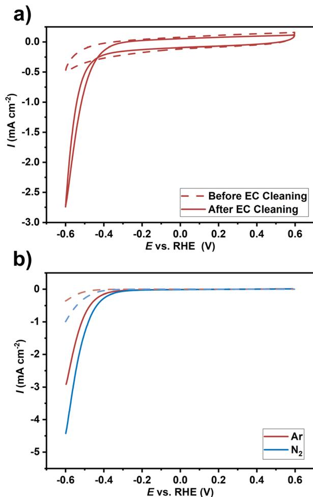
**Fig. 10** Electrochemical characterization of the ZrN-GC sample in 0.1 M sulfuric acid electrolyte with (a) showing the cyclic voltammety data before (dashed line) and after (solid line) electrochemical cleaning and (b) the difference in cyclic voltammety ( $10 \text{ mV s}^{-1}$ ) in Ar- (red) and  $\text{N}_2$  (blue)-saturated electrolyte. Shown is the backward scan of the 3<sup>rd</sup> scan. Dashed lines indicate background measurements of the glassy carbon substrate.
