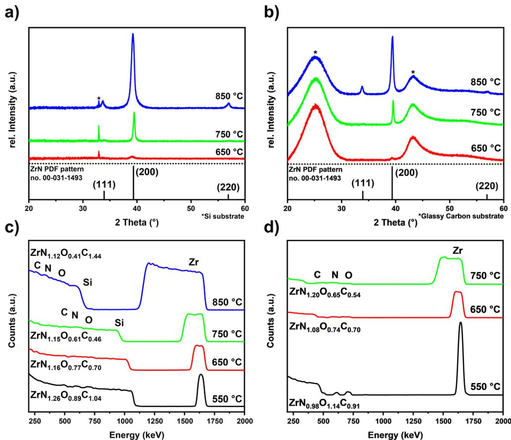
**Fig. 3** (a) and (b) XRD patterns of ZrN films deposited on Si and GC respectively as a function of substrate temperature. The XRD reference pattern of ZrN from PDF pattern no. 00-031-1493<sup>42</sup> are depicted in the respective patterns. (c) and (d) RBS analysis of ZrN films grown at different temperatures on Si and GC, respectively.
