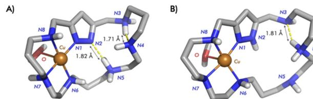
**Fig. 6** Representation of the most stable structure for the monoprotonated  $\text{Cu}^{2+}$ -L2 complex. (A)  $[\text{Cu}(\text{H}_2(\text{H}_{-1}\text{L2}))]^{4+}$  and (B)  $[\text{Cu}(\text{HL2})]^{4+}$ . Structure B is ca.  $25.3 \text{ kJ mol}^{-1}$  more stable than A.
