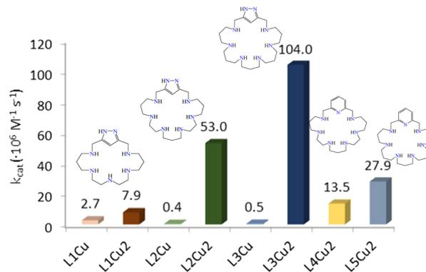
**Fig. 12** Plot of the *k*<sub>cat</sub> values for the mononuclear and binuclear Cu<sup>2+</sup>–**L1**, Cu<sup>2+</sup>–**L2**, Cu<sup>2+</sup>–**L3**, Cu<sup>2+</sup>–**L4** and Cu<sup>2+</sup>–**L5** systems.
