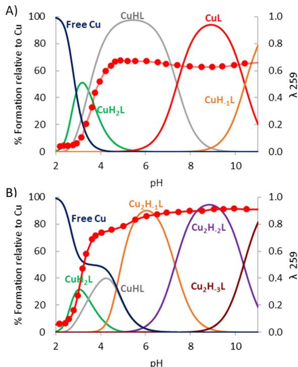
**Fig. 3** Distribution diagram for the system Cu<sup>2+</sup>–**L1** overlapped with the absorbance at 259 nm [**L1**] = 1 × 10<sup>–3</sup> M, (A) [Cu<sup>2+</sup>] = 1 × 10<sup>–3</sup> M and (B) [Cu<sup>2+</sup>] = 2 × 10<sup>–3</sup> M.
