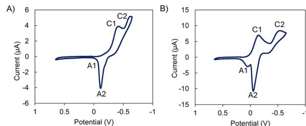
**Fig. 11** Cyclic voltammograms at the glassy carbon electrode for aqueous solution of the mononuclear (A) Cu–L1 and the binuclear (B)  $\text{Cu}_2\text{L1}$  systems,  $1 \times 10^{-4} \text{ M}$ , in 0.15 M NaCl at pH 7.0. Scan rate  $50 \text{ mV s}^{-1}$ .
