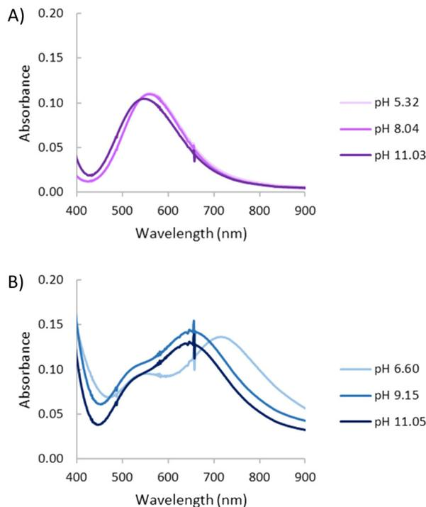
**Fig. 8** UV-Vis spectra for the system  $\text{Cu}^{2+}$ -L1 at variable pH. (A)  $[\text{Cu}^{2+}] = [\text{L1}] = 1 \times 10^{-3}$  M. (B)  $[\text{Cu}^{2+}] = 2 \times 10^{-3}$  M,  $[\text{L1}] = 1 \times 10^{-3}$  M.
