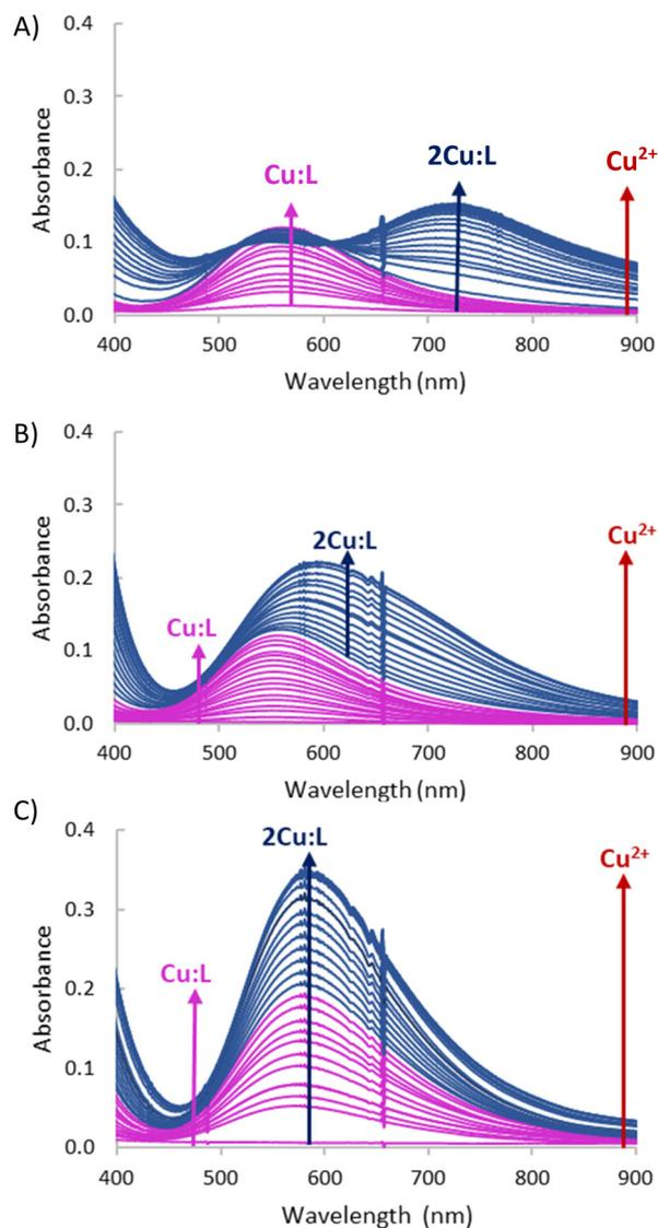
Fig. 7 Variation in the UV-Vis spectra of systems (A)  $\text{Cu}^{2+} : \text{L1}$ , (B)  $\text{Cu}^{2+} : \text{L2}$  and (C)  $\text{Cu}^{2+} : \text{L3}$  upon increasing additions of  $\text{Cu}^{2+}$  at pH = 6, the initial concentration of the ligands  $1 \times 10^{-3} \text{ M}$ .
