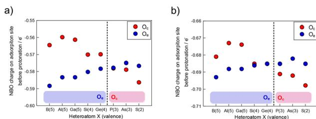
**Fig. 2** NBO charge on O<sub>c</sub> and O<sub>e</sub> without protonation in (a)  $\alpha$ -XMo<sub>12</sub> and (b)  $\alpha$ -XW. Red and blue plots represent NBO charge on O<sub>c</sub> and O<sub>e</sub>, respectively.
