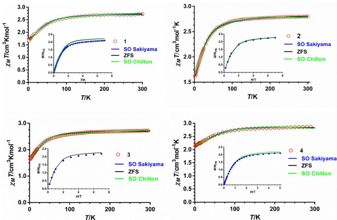
Fig. 5 Temperature dependence of  $\chi_M T$  (red circles) and field dependence of the magnetization at 2 K (inset, blue circles). Solid lines represent the best fit to eqn (1) (black line), (2) (green line) and (3) (blue line) with the parameters indicated in Table 1.
