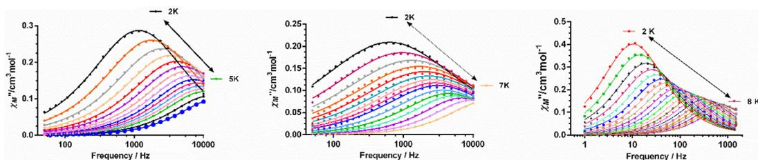
Fig. 7 Frequency dependence of the out-of-phase signals ( $\chi''_M$ ) at the indicated temperature ranges and under the optimal fields of 0.12 T for **2** (left) and **3** (centre) and 0.15 T (right) for **4**. Solid lines represent the best-fit curves to the generalized Debye model.
