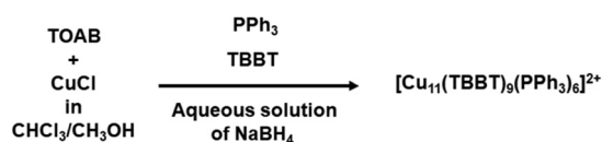
Fig. 6 Synthesis procedure of [\text{Cu}_{11}(\text{TBBT})_9(\text{PPh}_3)_6]^{2+} NC.
