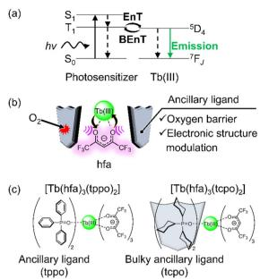
Fig. 1 (a) Excited-state dynamics of luminescent Tb(III) complexes with a small energy gap between T<sub>1</sub> and <sup>5</sup>D<sub>4</sub> levels (EnT: energy transfer, BEnT: back energy transfer). (b) Illustration of the strategy for highly luminescent Tb(III) complexes under air conditions. (c) Chemical structures of Tb(III) complexes used in this study.
