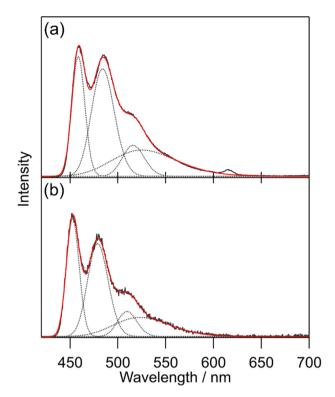
Fig. 4 Phosphorescence spectra ( $\lambda_{ex}$  = 350 nm, 100 K, under vacuum, delay = 20 ms) of the Gd(III) complexes (black lines): (a) [Gd(hfa)<sub>3</sub>(tppo)<sub>2</sub>] and (b) [Gd(hfa)<sub>3</sub>(tcpo)<sub>2</sub>] with peak deconvolution using the Gaussian function (dotted lines). The red lines are the summations of Gaussian functions.
