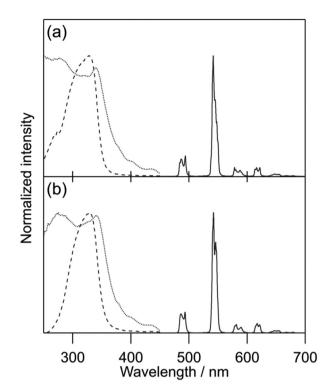
Fig. 3 Emission (solid line,  $\lambda_{\rm ex}$  = 360 nm), excitation (dotted line,  $\lambda_{\rm em}$  = 542 nm), and diffuse reflectance (dashed line) spectra of Tb(III) complexes in air: (a) [Tb(hfa)<sub>3</sub>(tppo)<sub>2</sub>] and (b) [Tb(hfa)<sub>3</sub>(tcpo)<sub>2</sub>].
