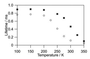
Fig. 5 Temperature-dependent emission lifetimes of  $[Tb(hfa)_3(tppo)_2]$  (circles) and  $[Tb(hfa)_3(tcpo)_2]$  (squares) ( $\lambda_{ex} = 356$  nm,  $\lambda_{em} = 542$  nm, under vacuum).
