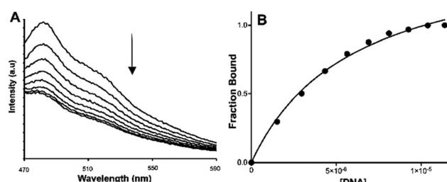
**Fig. 5** (A) Details of the luminescence response induced through progressive addition of 0.85  $\mu\text{M}$  of quadruplex folded HTS to complex **1**. (B) Binding curve for **1** with HTS constructed using emission data – continuous line shows fitting to binding to one-set-of-sites.
