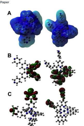
Fig. 2 Results of DFT calculations. (A) Electrostatic potential map of complexes  $\bf 1$  and  $\bf 2$ . (B) Calculated HOMO $-\bf 1$  of each complex. (C) Calculated LUMO $-\bf 1$  of each complex.
