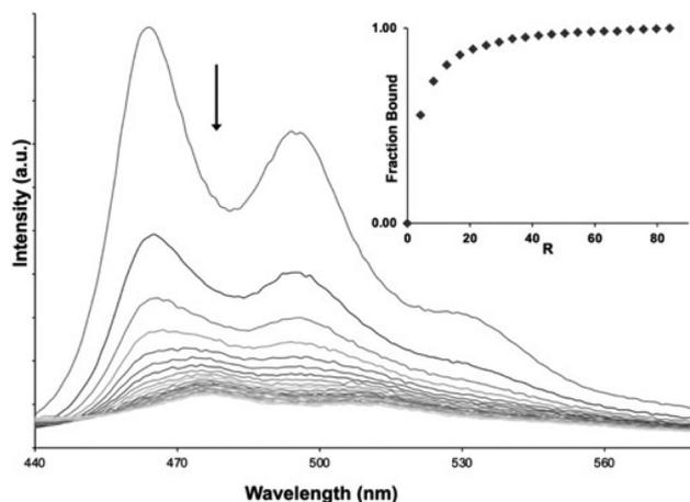
Fig. 3 Example of changes in the luminescence of a buffered aqueous 100 μM solution of **2** on addition of calf thymus-DNA, CT-DNA, up to excess. Inset: binding curve constructed from these data, *R* is the binding ratio.
