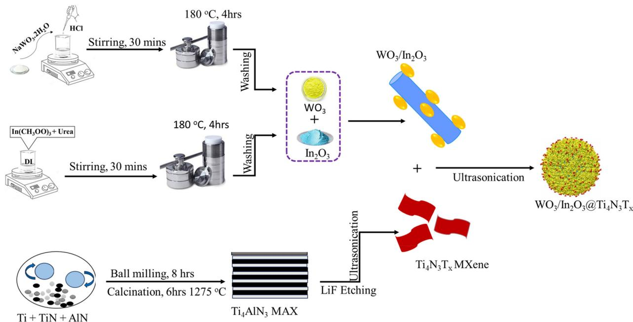
Fig. 1 Schematic of the synthesis of the  $\text{WO}_3/\text{In}_2\text{O}_3@ \text{Ti}_4\text{N}_3\text{T}_x$  composite.
