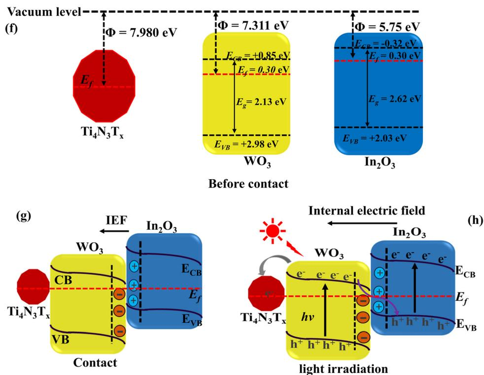
Fig. 11 Internal electric field and charge transfer.
