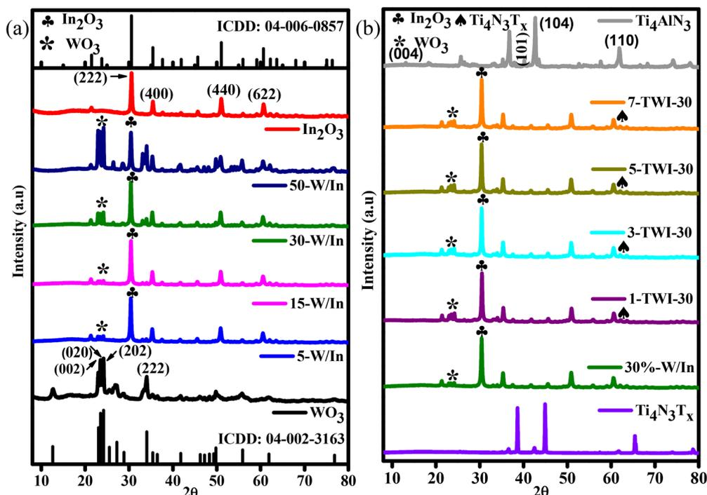
Fig. 2 XRD patterns for (a) pristine  $\text{WO}_3$ ,  $\text{In}_2\text{O}_3$ , and binary nanocomposites; (b)  $\text{Ti}_4\text{AlN}_3$  MAX,  $\text{Ti}_4\text{N}_3\text{T}_x$  MXene and ternary nanocomposites.
