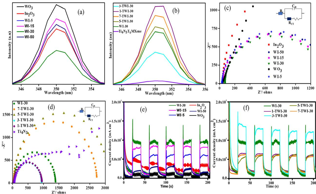
Fig. 8 (a and b) PL spectra, (c and d) EIS Nyquist plot of the as-prepared materials, inset: Randles–Ershler equivalent circuit. ( $C_{dl}$  = double layer capacitance,  $R_{CT}$  = charge transfer resistance, and  $R_s$  = solution resistance) and (e and f) photocurrent response of the pristine and nanocomposites.
