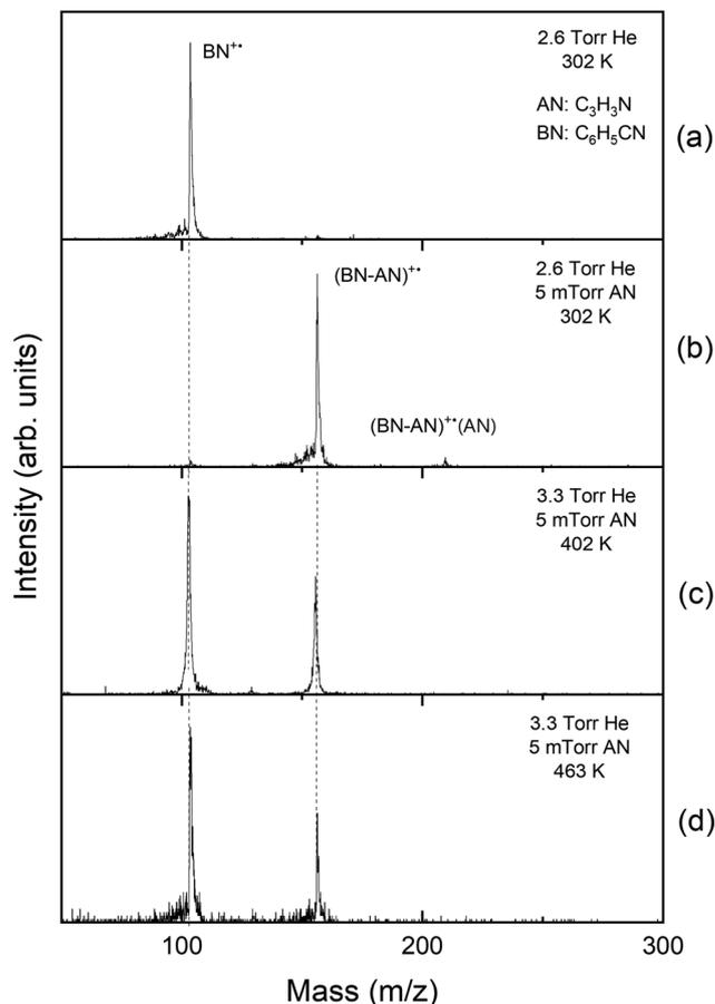
Fig. 1 Mass spectra obtained from the injection (19 eV) of the benzonitrile radical cation ( $BN^+$ ,  $C_6H_5CN$ ,  $m/z$  103) into: (a) a room temperature drift cell with 2.6 Torr He and no acrylonitrile (AN,  $C_3H_3N$ ,  $m/z$  53) and (b–d) with an acrylonitrile pressure of 5 mTorr at 302 K up to 463 K.
