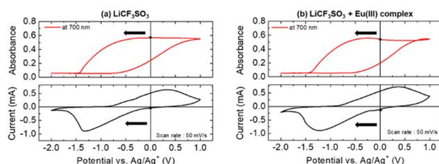
Fig. 1 Changes in the absorption at 700 nm (top) and the cyclic voltammogram (bottom) of the PB-modified electrode in PEG<sub>400</sub> electrolyte solution containing (a) LiCF<sub>3</sub>SO<sub>3</sub> (500 mM) and (b) LiCF<sub>3</sub>SO<sub>3</sub> (500 mM) and Eu(hfa)<sub>3</sub>(H<sub>2</sub>O)<sub>2</sub> (10 mM).
