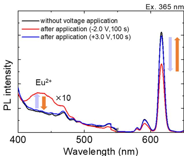
Fig. 5 Luminescence spectra from the ITO–PB device before and after applying reduction and oxidation voltages (reduction voltage:  $-2.0$  V for 100 s and oxidation voltage:  $+3.0$  V for 100 s). The excitation wavelength was 365 nm.
