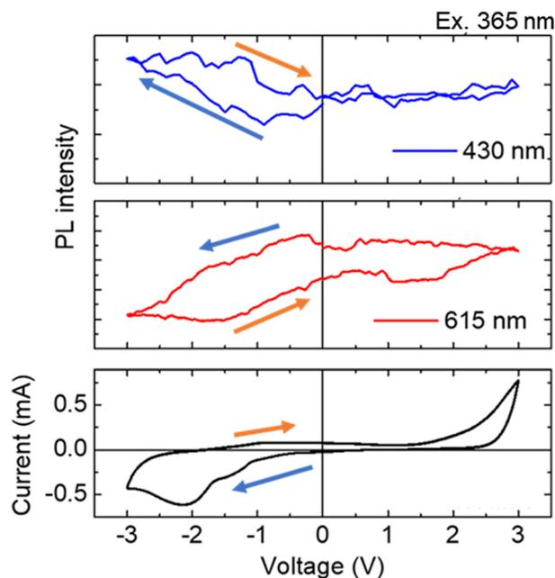
Fig. 7 Changes in the luminescence of  $\text{Eu}^{2+}$  at 430 nm (top) and  $\text{Eu}^{3+}$  at 615 nm (middle) during the cyclic voltammogram measurement (bottom) using the ITO–PB device. The excitation wavelength was 365 nm. The scan rate was  $100$   $\text{mV s}^{-1}$ .
