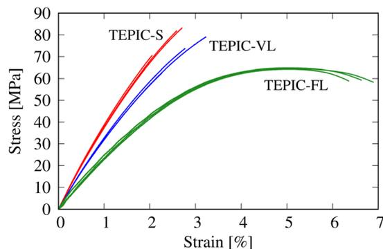
Fig. 8 Stress–strain curves in the uniaxial experiment.
