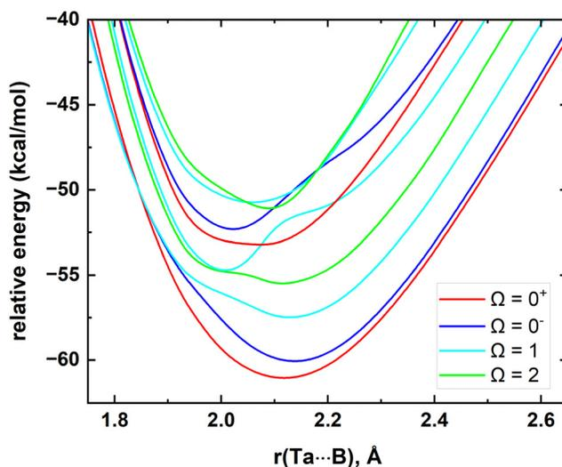
**Fig. 3** Low-lying spin-orbit coupling curves of TaB as a function of Ta...B distance [ $r(\text{Ta}\cdots\text{B})$ , Å]. The relative energies are referenced to the energy of the lowest  $\Omega$  state of Ta(<sup>4</sup>F) + B(<sup>2</sup>P) fragments at  $r = 200$  Å, which is set to 0 kcal mol<sup>-1</sup>. The  $\Omega = 0^+$ ,  $\Omega = 0^-$ ,  $\Omega = 1$ , and  $\Omega = 2$  curves are shown in red, blue, cyan, and green, respectively.
