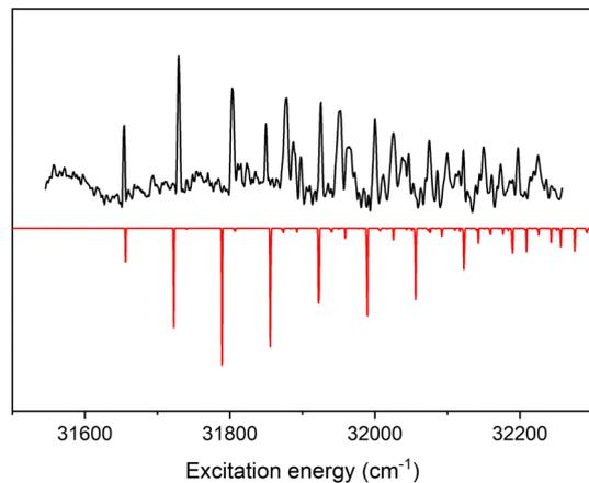
Fig. 7 Comparison of the depletion spectrum of  $N_1$ -methyl methyl urocanate excited at  $31653.1\text{ cm}^{-1}$  (see Fig. 6) with the Franck–Condon spectrum predicted for the  ${}^1\pi\pi^* \leftarrow S_0$  transition as obtained from TD-DFT calculations at the wB97XD/cc-pVDZ level and employing a scaling factor of 0.953 for the calculated vibrational frequencies.
