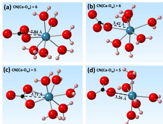
Fig. 4 Contact ion-pair formed at Ca to  $\text{O}_{\text{water}}$  CNs of (a), (b) 6 and (c), (d) 5 with 5 T of magnetic field. In each coordination environment, either bidentate or monodentate binding of  $\text{CO}_3^{2-}$  ion to  $\text{Ca}^{2+}$  was shown. Oxygen, hydrogen, carbon, and calcium atoms were shown as red, pink, black, and cyan spheres.
