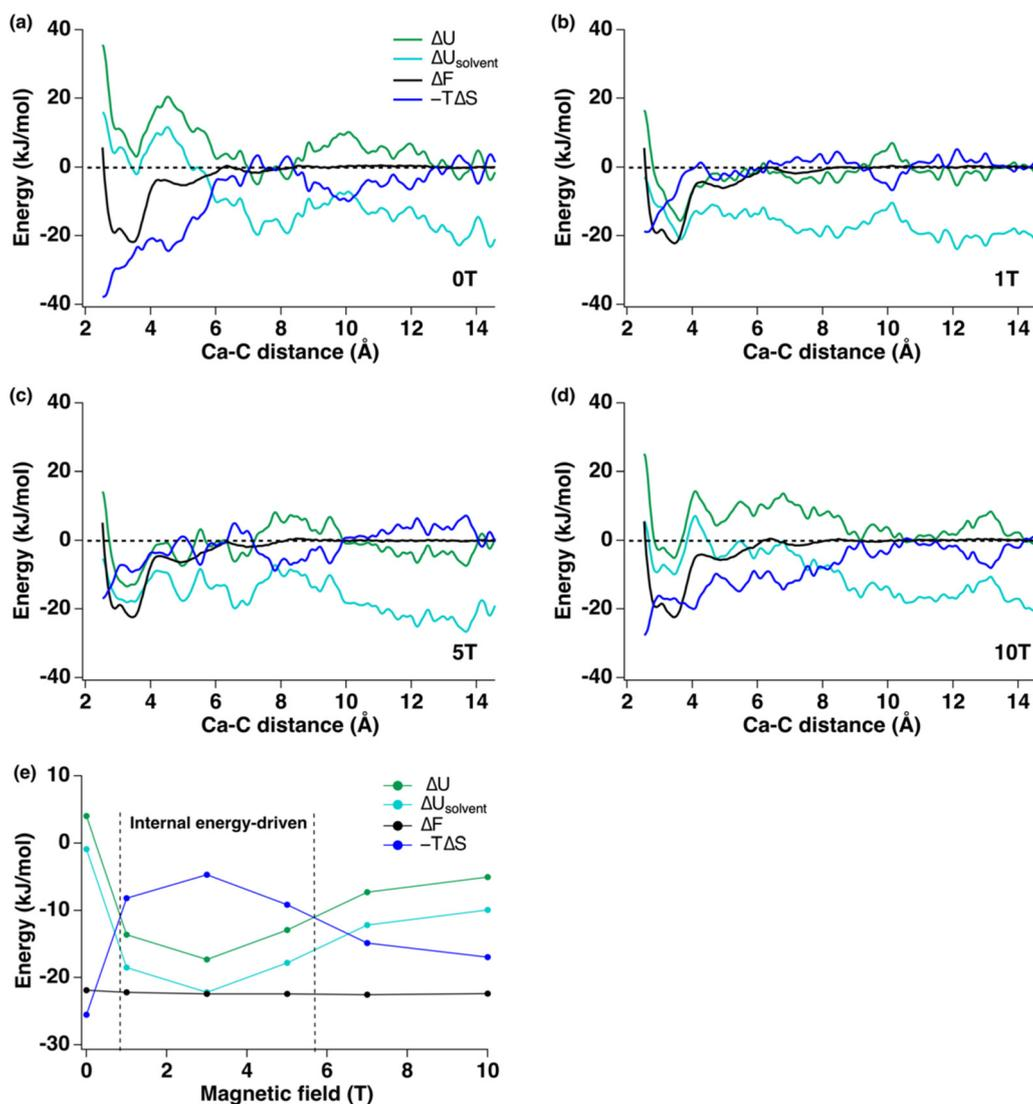
**Fig. 2** Deconvoluting the free energy ( $\Delta F$ ) into internal energy ( $\Delta U$ ), internal energy of solvent ( $\Delta U_{\text{solvent}}$ ), and entropic terms ( $-T\Delta S$ ) at 300 K under (a) 0 T, (b) 1 T, (c) 5 T, and (d) 10 T. (e) Changes in free energies and associated free energy components with magnetic fields from 0 T to 10 T.
