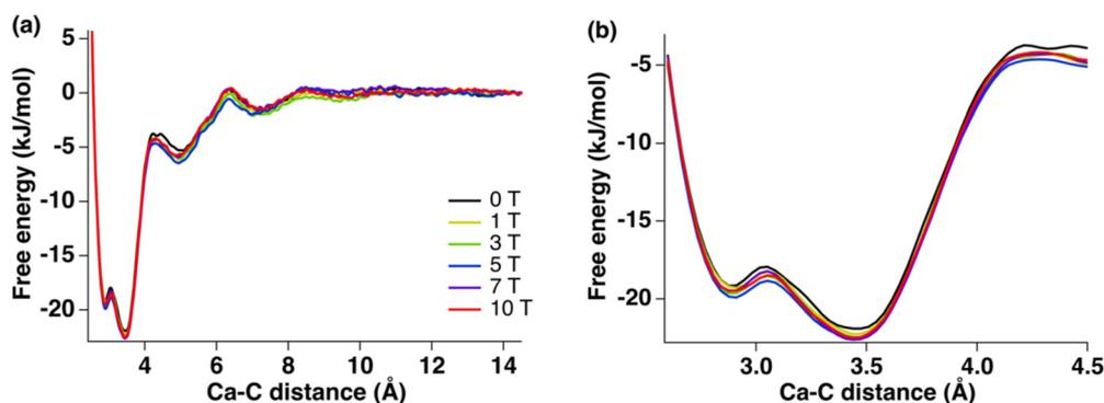
Fig. 1 (a) Free energy profiles of forming a [Ca–CO<sub>3</sub>]<sup>0</sup> ion-pair under a series of magnetic fields (0 T, 1 T, 3 T, 5 T, 7 T, and 10 T) at 300 K and (b) A zoomed-in view at the region where the contact ion-pair was formed.
