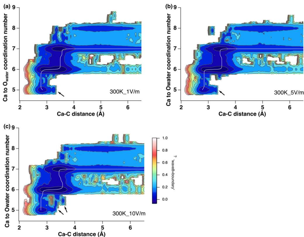
Fig. 7 The reweighted 2D free energy for the formation of  $[\text{Ca}-\text{CO}_3]^0$  ion pair at 300 K. Arrows indicated new structures formed as contact ion pairs under increasing electric field. The white lines indicated the minimum energy path.
