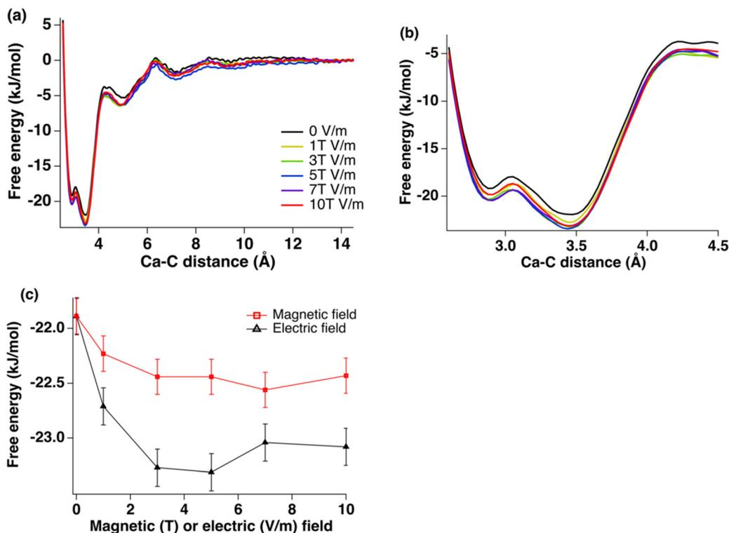
Fig. 5 (a) The free energy profiles of forming the  $[\text{Ca}-\text{CO}_3]^0$  ion-pair under a series of electric fields ( $0 \text{ V m}^{-1}$ ,  $1 \text{ V m}^{-1}$ ,  $3 \text{ V m}^{-1}$ ,  $5 \text{ V m}^{-1}$ ,  $7 \text{ V m}^{-1}$ , and  $10 \text{ V m}^{-1}$ ) at 300 K and (b) A zoomed-in view at the region where the contact ion-pair was formed. (c) Comparison in free energies ( $\Delta F$  in Tables 1 and 2) under increasing external field.
