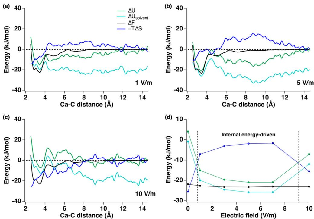
Fig. 6 Decomposition of the free energy ( $\Delta F$ ) as internal energy ( $\Delta U$ ), internal energy of solvent ( $\Delta U_{\text{solvent}}$ ), and entropic terms ( $-T\Delta S$ ) at 300 K under (a)  $1 \text{ V m}^{-1}$ , (b)  $5 \text{ V m}^{-1}$ , and (c)  $10 \text{ V m}^{-1}$ . (d) Changes in free energy and associated free energy components with electric fields.
