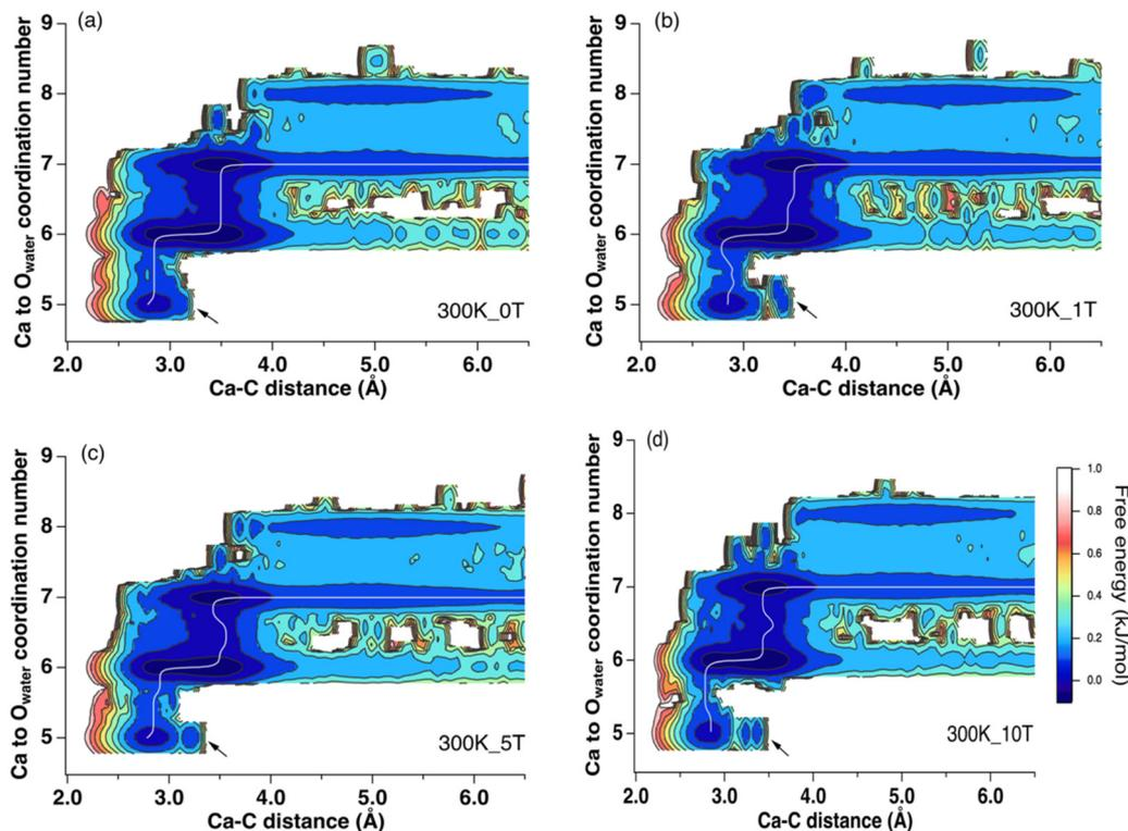
Fig. 3 The reweighted 2D free energy for the formation of  $[\text{Ca}-\text{CO}_3]^0$  ion-pair at 300 K. Arrows indicated new structures formed as contact ion-pairs under increasing magnetic fields. The white lines indicated the minimum energy path.
