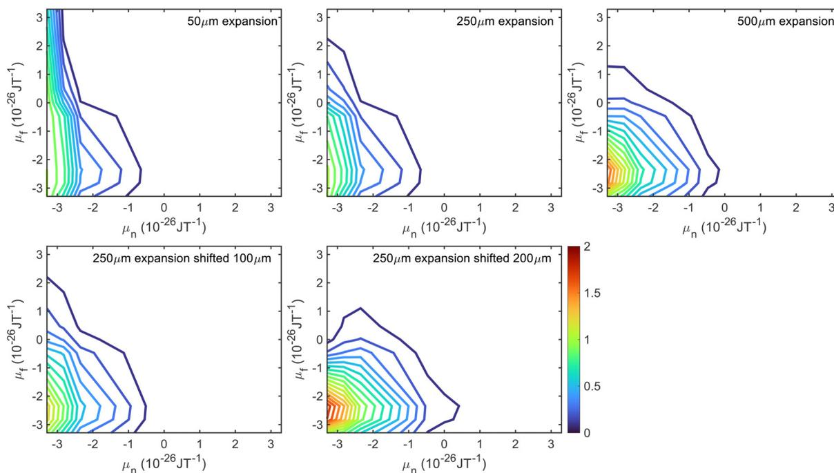
Fig. 2 Hexapole probabilities calculated using the trajectory calculations described in the text for  $\text{H}_2$  travelling at a velocity of 1470  $\text{m s}^{-1}$  for a 50  $\mu\text{m}$  expansion (top left), 250  $\mu\text{m}$  expansion (top middle), 500  $\mu\text{m}$  expansion (top right), 250  $\mu\text{m}$  expansion shifted by 100  $\mu\text{m}$  (bottom left) and 250  $\mu\text{m}$  expansion shifted by 200  $\mu\text{m}$  (bottom middle).
