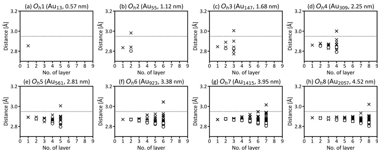
Fig. 2 Calculated intralayer Au–Au bond lengths [Å] in gold nanoparticles with (a) 13 ( $O_h1$ ), (b) 55 ( $O_h2$ ), (c) 147 ( $O_h3$ ), (d) 309 ( $O_h4$ ), (e) 561 ( $O_h5$ ), (f) 923 ( $O_h6$ ), (g) 1415 ( $O_h7$ ), and (h) 2057 ( $O_h8$ ) atoms. The x-axes correspond to the indices of the layers in the nanoparticles. Black dotted lines correspond to the bond length in the bulk fcc gold crystal.
