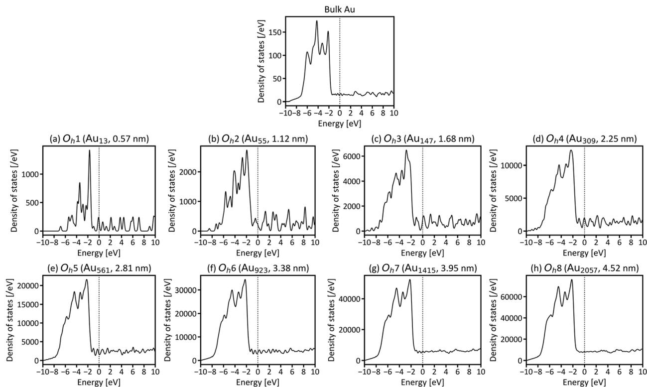
**Fig. 3** Total density of states (DOS) for gold nanoparticles with (a) 13 ( $O_h1$ ), (b) 55 ( $O_h2$ ), (c) 147 ( $O_h3$ ), (d) 309 ( $O_h4$ ), (e) 561 ( $O_h5$ ), (f) 923 ( $O_h6$ ), (g) 1415 ( $O_h7$ ), and (h) 2057 ( $O_h8$ ) atoms ( $E_F$  is set to be zero). The DOS of bulk fcc gold is provided at the top for comparison. Note that the present total DOS is defined for the whole system, not per atom.
