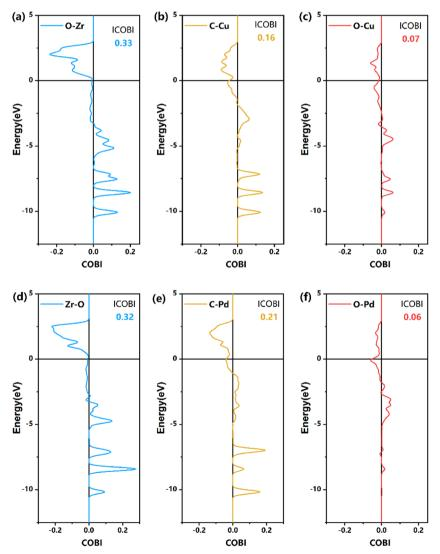
Fig. 7 COBI analysis of the bonding nature and strength of TS1 on the formate pathway, as shown in Fig. 6. (a)-(c) Z/CuPd(100)-Cu, (d)-(f) Z/CuPd(100)-Pd.
