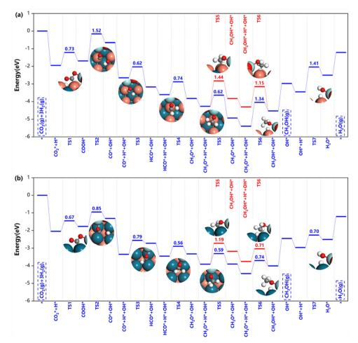
Fig. 8 Potential energy diagrams and corresponding transition state structures of methanol formation over (a) Z/CuPd(100) - Cu and (b) Z/CuPd(100) -Pd on the RWGS + CO-hydro pathway
