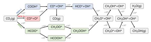
Fig. 5 Reaction network for  $CO_2$  hydrogenation to methanol and carbon monoxide over  $Zr_3O_6/CuPd$  inverse catalysts. PATH II: formate, PATH III: RWGS + CO-hydro, PATH III:  $CO_2$  direct activation.
