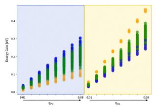
Fig. 8 Energy gain per atom for AuPd in various environments w.r.t. the vacuum varying the strength of Pd (blue shadow)/Au (yellow shadow) interaction  $(\eta_{\alpha})$ , fixing  $\rho_{\alpha}$  at 1.5. Orange circles represent core-shell initial configurations, mixing configurations are in blue and Janus-like in green. An inversion of the chemical ordering stability occurs as soon as only Pd interacts while AuPd favours core (Pd)-shell (Au) ordering
