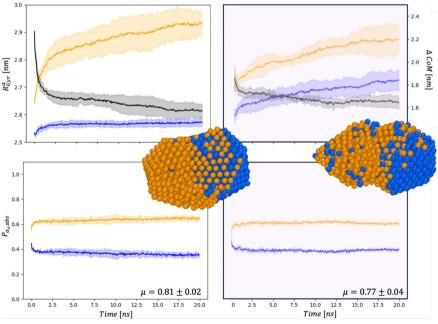
Fig. 5 Chemical distribution for  $\text{Au}_{561}^{\text{lh}} - \text{Pd}_{561}^{\text{lh}}$  in a vacuum (right) and and in set34 (right) for  $R_{\text{gyr}}^{\alpha}$  in nm and  $\Delta \text{CoM}$  in nm (top), and  $P_{\alpha,\text{abs}}$  (bottom). Snapshots are taken after 20 ns with the same colour-coding as in Fig. 4.
