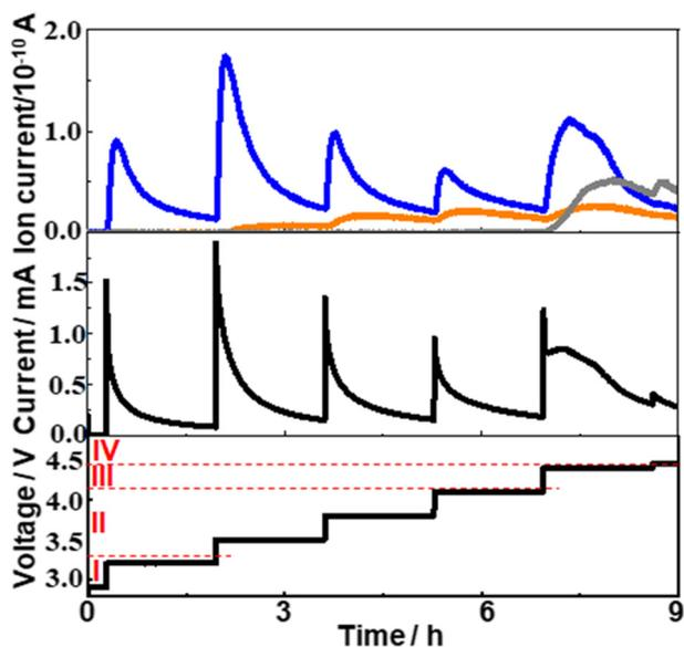
Fig. 5 Time dependencies of current (middle panel) and mass signal of  $m/z = 18$  (orange), 32 (blue), and 44 (gray) (top panel) when the sequences of the voltage step (300 mV step and 6000 s stay before the next step) were applied as shown in the bottom panel.
