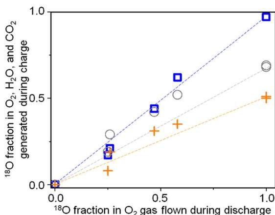
Fig. 11 Fractions of  $^{18}\text{O}$  in  $\text{O}_2$  ( $\square$ ),  $\text{H}_2\text{O}$  ( $+$ ), and  $\text{CO}_2$  ( $\circ$ ) generated during charge as a function of the fraction of  $^{18}\text{O}$  in the  $\text{O}_2$  gas flow during discharge.
