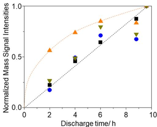
Fig. 8 Discharge time dependencies of integrated signal intensities, *i.e.*, current ( $\blacktriangledown$ ), and ion current of  $m/z = 18$  ( $\blacktriangle$ ),  $32$  ( $\bullet$ ), and  $44$  ( $\blacksquare$ ), normalized by those of 9.6 h discharge.
