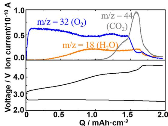
Fig. 2 Typical discharge/charge curves (bottom panel) and ion currents of the Q-mass at  $m/z = 18$  ( $H_2O$ ), 32 ( $O_2$ ), and 44 ( $CO_2$ ) during charge (top panel) of a Li/TEGDME-1M LiTFSI/KJCNT cell (electrode area:  $2 \text{ cm}^2$ ) obtained under a constant current of  $0.4 \text{ mA}$  ( $0.2 \text{ mA cm}^{-2}$ ).
