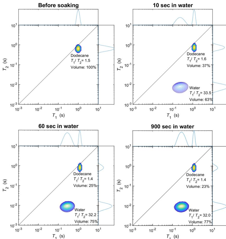
Fig. 4  $T_1$ - $T_2$  maps of the alumina pellet at four different time steps during an imbibition experiment. Initially, only one peak is present, representing the hydrocarbon phase. After soaking the pellet in water, a second peak appears, whose volume increases at longer soaking times.
