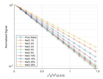
Fig. 2 Stejskal-Tanner plot for brines of different salinities within the pores of alumina pellets. The solid lines represent exponential fits using egn (6)
