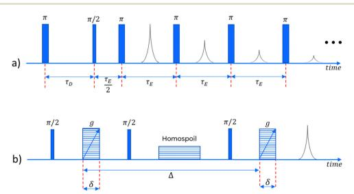
Fig. 1 (a) The IR-CPMG pulse sequence, which is repeated for several different values of delay time  $(\tau_D)$  while the echo time  $(\tau_E)$  remains constant. (b) The PGSTE pulse sequence, repeated for several different magnitudes of magnetic field gradient (g). The duration of the gradient pulses is  $\delta$ , and the time interval between those pulses is  $\Delta$ . Striped boxes represent gradient pulses, along the direction of the external field
