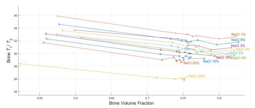
Fig. 6 Plot showing the  $T_1/T_2$  ratio of the ten different brine samples, versus the volume fraction of the same brines during one set of the imbibition experiments. Each data point represents a different time step, with the leftmost points representing 10 seconds of soaking time and the rightmost point representing a week of soaking, for each salinity. The solid lines connecting the data points act as a guide to the eye.
