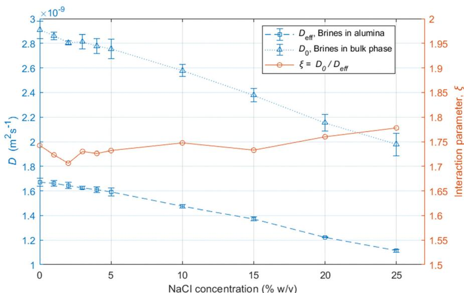
Fig. 3 Diffusion coefficients and  $\xi$  values versus salinity, for NaCl brines in mixed-phase alumina pellets. Error bars were calculated from the standard deviations between three iterations of the same measurements, using different pellets. All the lines between data points are a guide to the eye, not fittings.
