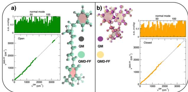
**Fig. 5** (a) Open conformer: overlap between QM (gray solid spheres) and QMD-FF (transparent green spheres) optimized geometries (right) and comparison of QM and QMD-FF frequencies and normal mode overlap (left). (b) Closed conformer: overlap between QM (purple solid spheres) and QMD-FF (transparent orange spheres) optimized geometries (left) and comparison of QM and QMD-FF frequencies and normal mode overlap (right).
