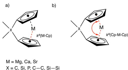
Fig. 4 Special force constants used in this work. (a) Local force constant between the metal (M) and geometric centerpoint of the Cp ring  $k^l(\text{M-Cp})$ . (b) Local force constant between the Cp-M-Cp angle  $k^l(\text{Cp-M-Cp})$ .
