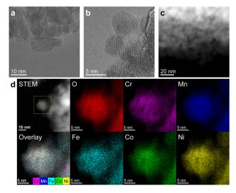
**Fig. 3** High-resolution TEM images (a and b), HAADF-STEM image (c), and STEM and EDX mappings (d) of HE-MARIMO. An overlay image in (d) created by merging EDX mapping images of Cr, Mn, Fe, Co, and Ni.
