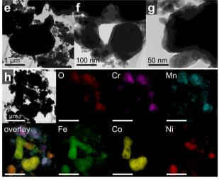
Fig. 5 TEM images (a–c), STEM and EDX mapping images (d) of the spent HE-MARIMO. Scale bars of EDX mapping images (d) are 500 nm. TEM images (e–g), and STEM and EDX mapping images (h) of spent sss-composite. Scale bars of EDX mapping images (h) are 2  $\mu$ m.
