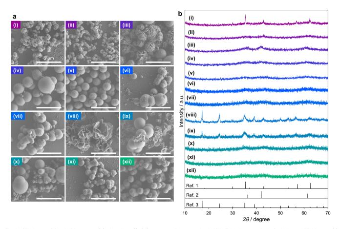
Fig. 1 SEM images (a) and XRD patterns (b) of products (i)–(xii) corresponding to entries 1–12 in Table 1, respectively. Scale bars of SEM images (a) are 5  $\mu$ m. Black lines in (b), ref. 1, 2, and 3, correspond to reference diffraction peak positions of cubic Fe<sub>3</sub>O<sub>4</sub> (PDF#00-001-1111), cubic FeO (PDF#00-001-1223), and cubic Co(Fe(CN)<sub>5</sub>NO)·5H<sub>2</sub>O (PDF#00-043-0768), respectively.
