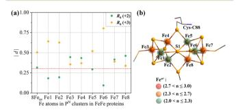
Fig. 3 (a) The weighted average |d| values of 8Fe<sub>av</sub> and Fe1-Fe8 atoms in P<sup>N</sup> clusters (PDB codes: 8BOQ and 8OIE) calculated from  $R_0$  (+2) and  $R_0$  (+3). Red dashed lines represent D = 0.3. (b) The valence distributions of Fe atoms in PN clusters of FeFe proteins.
