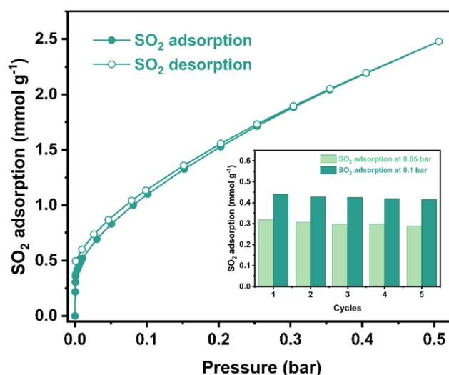
**Fig. 2** Experimental  $\text{SO}_2$  adsorption–desorption isotherm collected for a fully activated  $[\text{NiSi}]@\text{NU-1000}$  sample (filled green diamonds = adsorption; open green diamonds = desorption) at 298 K and up to 0.5 bar. Inset: adsorption–desorption cycles for  $\text{SO}_2$  in  $[\text{NiSi}]@\text{NU-1000}$  at 0.05–0.1 bar and 298 K. The reactivation step was carried out only by applying vacuum ( $1.7 \times 10^{-3}$  torr) for 45 minutes at room temperature (298 K).
