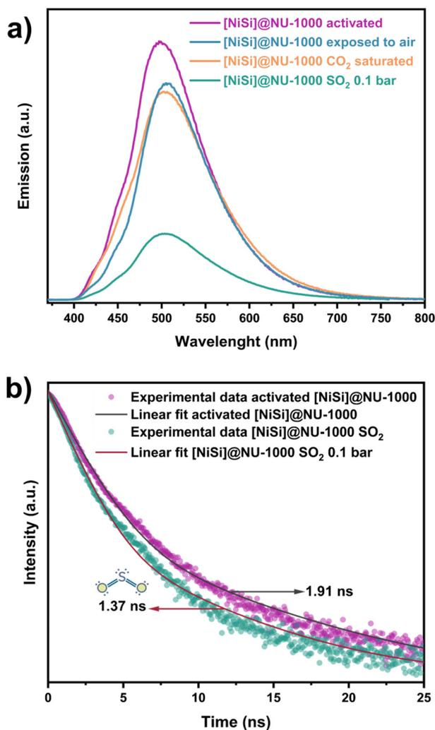
**Fig. 3** (a) Solid-state emission spectra of activated [NiSi]@NU-1000 (purple line), and after exposure to 0.1 bar of SO<sub>2</sub> (green line), CO<sub>2</sub> (orange line), and air (blue line). The excitation wavelength was set at 350 nm, (b) time-resolved photoluminescence decay spectra of activated [NiSi]@NU-1000, and after exposure to 0.1 bar of SO<sub>2</sub> measured at 335.6 nm excitation and at 500 nm emission.
