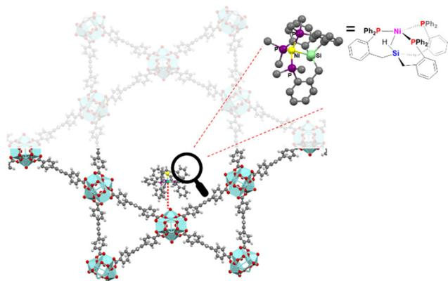
**Fig. 1** Structure representation of NU-1000 post-synthetically grafted with a nickel phosphinosilyl complex. Atom label: light blue: Zr, yellow: Ni, dark grey: carbon, light grey: hydrogen, purple: P and green: Si.
