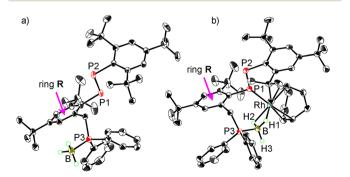
Fig. 2 Molecular structures of (a) diphosphene-phosphineborane ligand 1 and (b) diphosphene-rhodium complex 7. Thermal ellipsoids are drawn at 50% probability. Hydrogen atoms except BH<sub>3</sub>, anion BF<sub>4</sub>, and solvated dichloroethanes in 7 are omitted for clarity.
