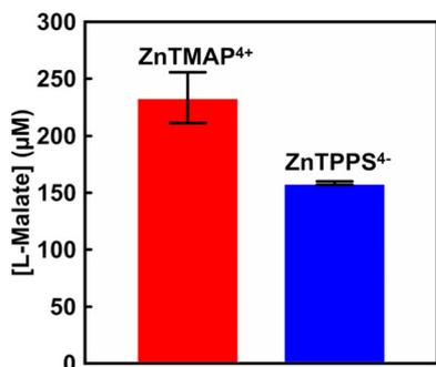
**Fig. 4** The concentration of L-malate production in the system of sodium pyruvate, magnesium chloride, TEOA, [Cp\*Rh(bpy)(H<sub>2</sub>O)]<sup>2+</sup>, NAD<sup>+</sup>, MDH and CO<sub>2</sub> gas in the presence of ZnTMAP<sup>4+</sup> (red) or ZnTPPS<sup>4-</sup> (blue) after 5 h irradiation. Errors were obtained from the average of multiple trials.
