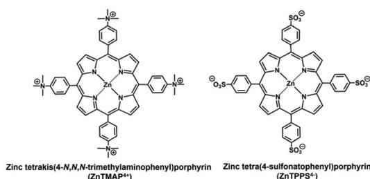
Fig. 2 Chemical structures of zinc tetrakis(4-N,N,N-trimethylaminophenyl)porphyrin (ZnTMAP<sup>4+</sup>) and zinc tetra(4-sulfonatophenyl)porphyrin (ZnTPPS<sup>4-</sup>).
