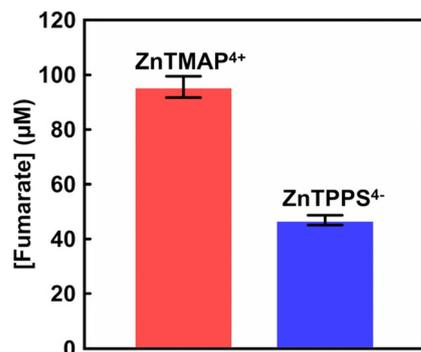
**Fig. 5** The concentration of fumarate production in the system of sodium pyruvate, magnesium chloride, TEOA,  $[\text{Cp}^*\text{Rh}(\text{bpy})(\text{H}_2\text{O})]^{2+}$ ,  $\text{NAD}^+$ , MDH, FUM and  $\text{CO}_2$  gas in the presence of  $\text{ZnTMAP}^{4+}$  (red) or  $\text{ZnTPPS}^{4-}$  (blue) after 5 h irradiation. Errors were obtained from the average of multiple trials.
