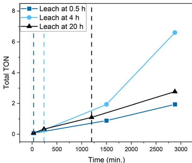
**Fig. 10** Leaching test data for UiO-67-[1Cu][BF<sub>4</sub>]<sub>2</sub>. MOF separated from solution at 0.5 h (dark blue line), at 4 h (light blue line), and at 20 h (black line) contact time and left reacting until 48 h total reaction time.
