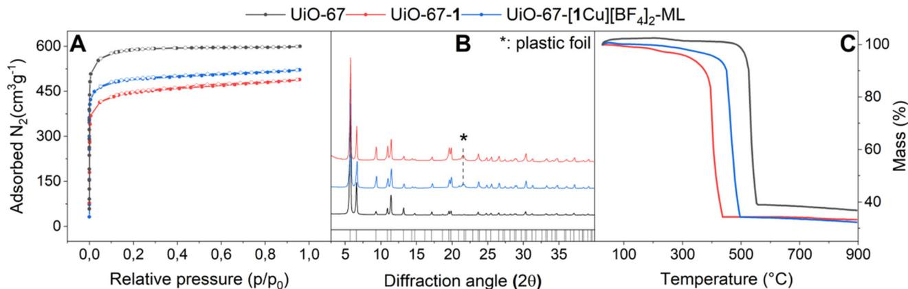
**Fig. 3** Basic characterization of UiO-67 (black), UiO-67-1 (blue) and UiO-67-[1Cu][BF<sub>4</sub>]<sub>2</sub>-ML (red). (A) Nitrogen adsorption isotherms performed at 77 K. (B) Measured powder X-ray diffractograms (Y-axis: normalized intensity), with calculated reflections given in the rug. (C) Thermogravimetric analysis (30 °C – 900 °C) performed in synthetic air (100 mLmin<sup>-1</sup>).
