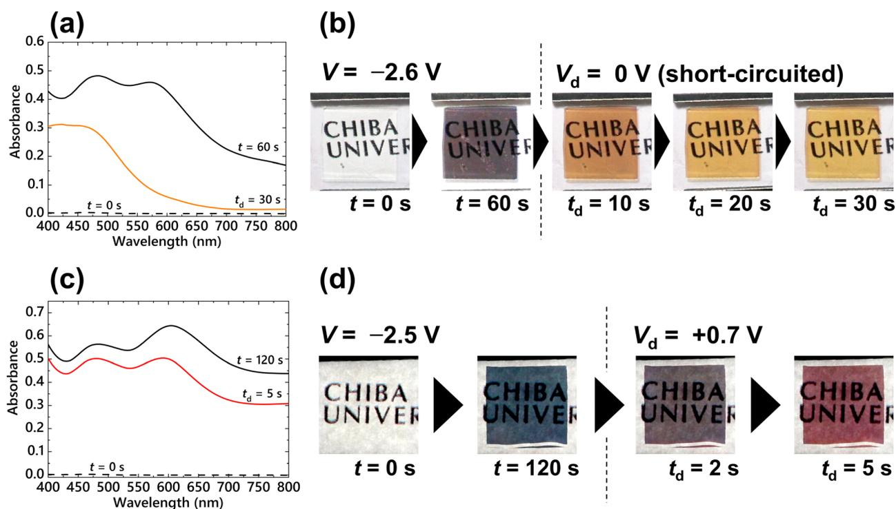
Fig. 8 The absorption spectra (a) and device images (b) of P-ECD during voltage application ( $V = -2.6$  V,  $t = 60$  s,  $V_d = 0$  V,  $t_d = 30$  s). The absorption spectra (c) and device images (d) of P-ECD during voltage application ( $V = -2.5$  V,  $t = 120$  s,  $V_d = +0.7$  V,  $t_d = 5$  s).
