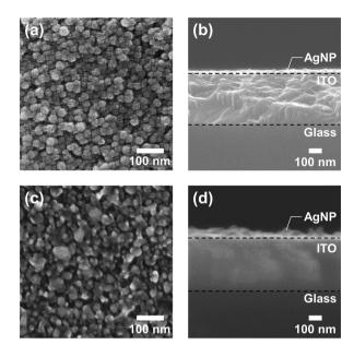
Fig. 6 FE-SEM images of the surface (a) and cross-section (b) of the P-ECD electrode where AgNPs were electrodeposited after a constant voltage application (V = -2.5 V, t = 120 s). FE-SEM images of the surface (c) and cross-section (d) of the B-ECD electrode where AgNPs were electrodeposited after a step voltage application ( $V_1 = -3.5 \text{ V}, t_1 =$ 100 ms,  $V_2 = -1.6$  V,  $t_2 = 60$  s).
