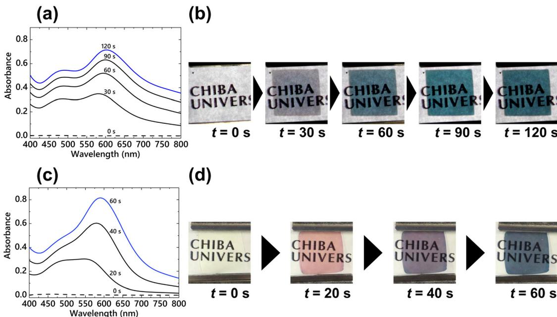
Fig. 5 The change of absorption spectra (a) and device images (b) of the P-ECD during constant voltage application ( $V = -2.5$  V,  $t = 120$  s). The change of absorption spectra (c) and device images (d) of the B-ECD during step voltage application ( $V_1 = -3.5$  V,  $t_1 = 100$  ms,  $V_2 = -1.6$  V,  $t_2 = 60$  s).
