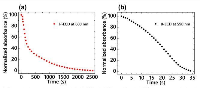
Fig. 7 Change in absorbance at the peak wavelength in Fig. 5 (at 600 nm for P-ECD and at 590 nm for B-ECD) after applying cyan coloration voltage ((a) P-ECD: V = -2.5 V, t = 120 s and (b) B-ECD:  $V_1 = -3.5 \text{ V}$ ,  $t_1 = 100 \text{ ms}$ ,  $V_2 = -1.6 \text{ V}$ ,  $t_2 = 60 \text{ s}$ ). The absorbance at each wavelength was normalized to 100% at the end of the voltage application.
