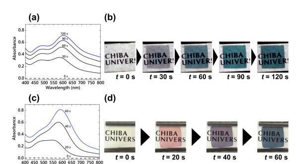
Fig. 5 The change of absorption spectra (a) and device images (b) of the P-ECD during constant voltage application (V = -2.5 V, t = 120 s). The change of absorption spectra (c) and device images (d) of the B-ECD during step voltage application ( $V_1 = -3.5 \text{ V}$ ,  $t_1 = 100 \text{ ms}$ ,  $V_2 = -1.6 \text{ V}$ ,  $t_2 = 60 \text{ s}$ ).
