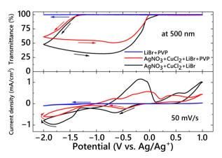
Fig. 1 Change in transmittance at 500 nm (top) and cyclic voltammogram (bottom) of the three-electrode EC cell with various EC electrolytes (blue: LiBr and PVP in DMSO; red: AgNO<sub>3</sub>, CuCl<sub>2</sub>, LiBr, and PVP in DMSO; black: AgNO<sub>3</sub>, CuCl<sub>2</sub>, and LiBr in DMSO).
