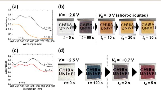
Fig. 8 The absorption spectra (a) and device images (b) of P-ECD during voltage application (V = -2.6 V, t = 60 s,  $V_d = 0 \text{ V}$ ,  $t_d = 30 \text{ s}$ ). The absorption spectra (c) and device images (d) of P-ECD during voltage application (V = -2.5 V, t = 120 s,  $V_d = +0.7 \text{ V}$ ,  $t_d = 5 \text{ s}$ ).
