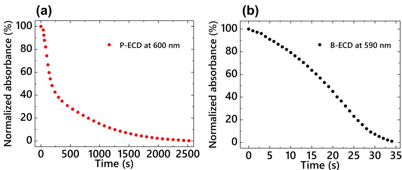
Fig. 7 Change in absorbance at the peak wavelength in Fig. 5 (at 600 nm for P-ECD and at 590 nm for B-ECD) after applying cyan coloration voltage ((a) P-ECD:  $V = -2.5$  V,  $t = 120$  s and (b) B-ECD:  $V_1 = -3.5$  V,  $t_1 = 100$  ms,  $V_2 = -1.6$  V,  $t_2 = 60$  s). The absorbance at each wavelength was normalized to 100% at the end of the voltage application.
