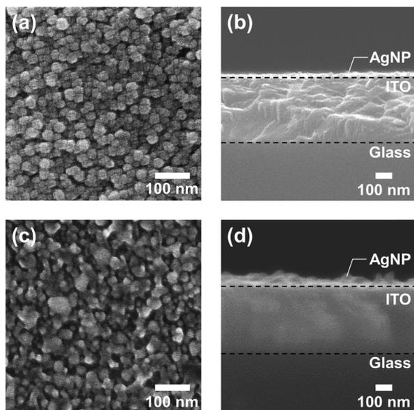
Fig. 6 FE-SEM images of the surface (a) and cross-section (b) of the P-ECD electrode where AgNPs were electrodeposited after a constant voltage application ( $V = -2.5$  V,  $t = 120$  s). FE-SEM images of the surface (c) and cross-section (d) of the B-ECD electrode where AgNPs were electrodeposited after a step voltage application ( $V_1 = -3.5$  V,  $t_1 = 100$  ms,  $V_2 = -1.6$  V,  $t_2 = 60$  s).
