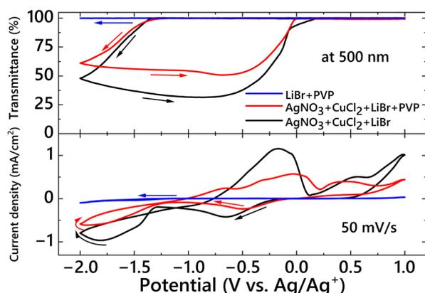
Fig. 1 Change in transmittance at 500 nm (top) and cyclic voltammogram (bottom) of the three-electrode EC cell with various EC electrolytes (blue: LiBr and PVP in DMSO; red:  $\text{AgNO}_3$ ,  $\text{CuCl}_2$ , LiBr, and PVP in DMSO; black:  $\text{AgNO}_3$ ,  $\text{CuCl}_2$ , and LiBr in DMSO).
