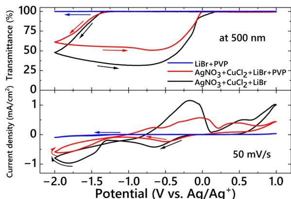
Fig. 1 Change in transmittance at 500 nm (top) and cyclic voltammogram (bottom) of the three-electrode EC cell with various EC electrolytes (blue: LiBr and PVP in DMSO; red:  $\text{AgNO}_3$ ,  $\text{CuCl}_2$ , LiBr, and PVP in DMSO; black:  $\text{AgNO}_3$ ,  $\text{CuCl}_2$ , and LiBr in DMSO).
