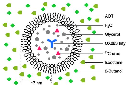
Fig. 3 Schematic of the reverse-micelle system, emulating the PA delivered close to the target molecule ( $^{13}\text{C}$ -urea). The positions (inside or outside the reverse micelle) of each type of molecule used to prepare the reverse-micelle sample are shown in the figure.
