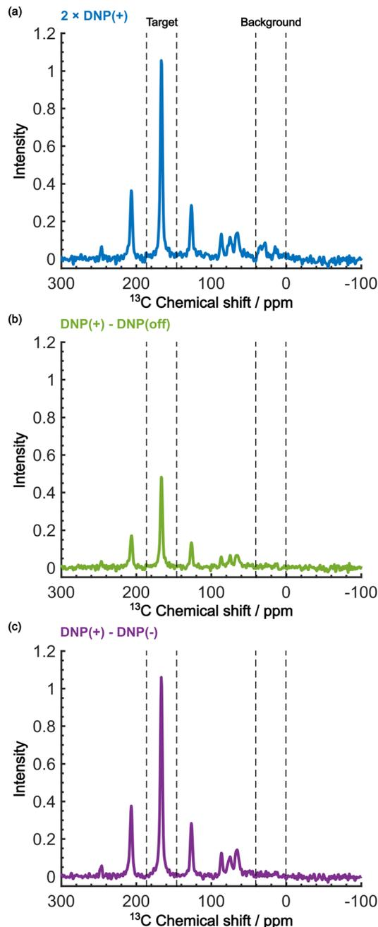
Fig. 6 Demonstration of background signal suppression at  $\tau = 60$  s. The DNP-enhanced spectra with (a) the positive DNP, (b) the MW-off data subtraction, and (c) the Oops treatment are shown. The data in (a) are the same as in Fig. 5b (blue, an average of two scans), but were vertically scaled by a factor of 2 for direct comparability in the same total experimental time.
