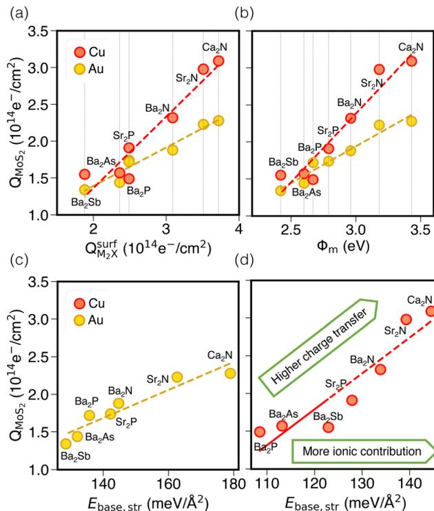
Fig. 3 (a) Correlation of  $Q_{\text{MoS}_2}$  and  $Q_{\text{M}_2\text{X}}^{\text{surf}}$  in Au and Cu-based interfaces. (b) Correlation of  $Q_{\text{MoS}_2}$  and the monolayer electrene work function ( $\Phi_{\text{m}}$ ). Also shown are correlations between the base-functional (ionic) component of the exfoliation energy and  $Q_{\text{MoS}_2}$  for Au (c) and Cu (d) interfaces, respectively.
