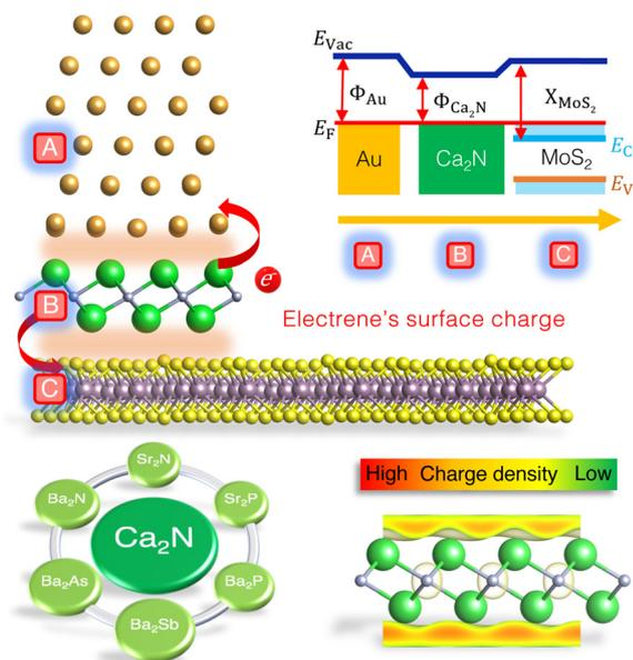
Fig. 1 Top: Schematic design of the Au/MoS<sub>2</sub> interface with monolayer Ca<sub>2</sub>N as an intermediate layer. The associated band diagram indicates the removal of the Schottky barrier upon metallization of the MoS<sub>2</sub> bands. Bottom: List of all stable M<sub>2</sub>X electrides, along with a 3D representation of the electrene's surface charge.
