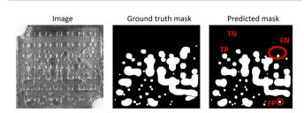
Fig. 4 Demonstration of an optical image along with the ground truth and predicted masks. Examples of true-positive (TP), true-negative (TN), false-positive (FP), and false-negative (FN) predictions are shown on the predicted mask
