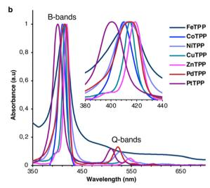
Fig. 1 (a) Synthesis of MTPPs from TPP. (b) Normalized UV/Vis absorption spectra of MTPPs in CH2Cl2 at rt.
